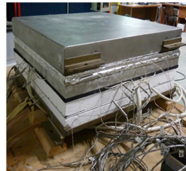
Fig. 5. Illustrative chart and general view of Perugia guarded hot plate.
