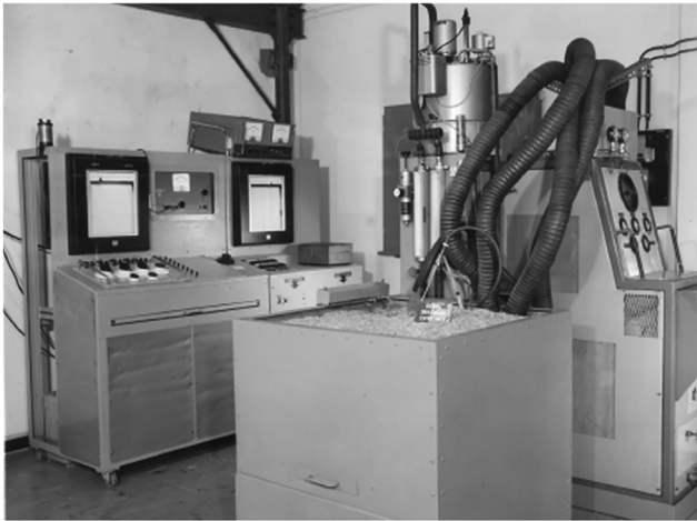
Fig. 18. Guarded hot plate of LNE in 1962.
