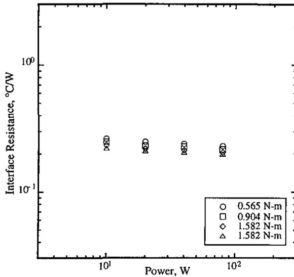
Figure 7 Interface resistance as a function of module power dissipation for Type III anodized SEM-E frame guide rib to Type II anodized chassis card rail.
