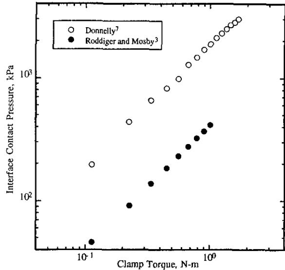
Figure 4 Comparison of the interface contact pressure as a function of wedge clamp torque from Roddiger and Mosby<sup>3</sup> and Donnelly<sup>7</sup>.
