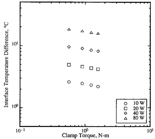
Figure 12 Interface temperature difference as a function of clamp torque for Type III anodized SEM-E frame guide rib to Type II anodized chassis card rail.
