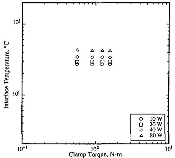
Figure 10 Interface temperature as a function of clamp torque for Type III anodized SEM-E frame guide rib to Type II anodized chassis card rail.
