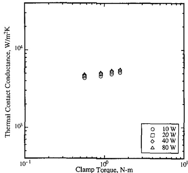
Figure 6 Thermal contact conductance as a function of clamp torque for Type III anodized SEM-E frame guide rib to Type II anodized chassis card rail.
