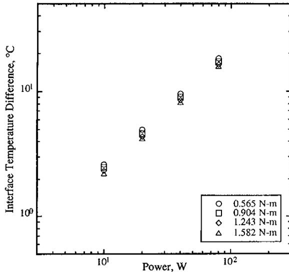
Figure 11 Interface temperature difference as a function of module power dissipation for Type III anodized SEM-E frame guide rib to Type II anodized chassis card rail.
