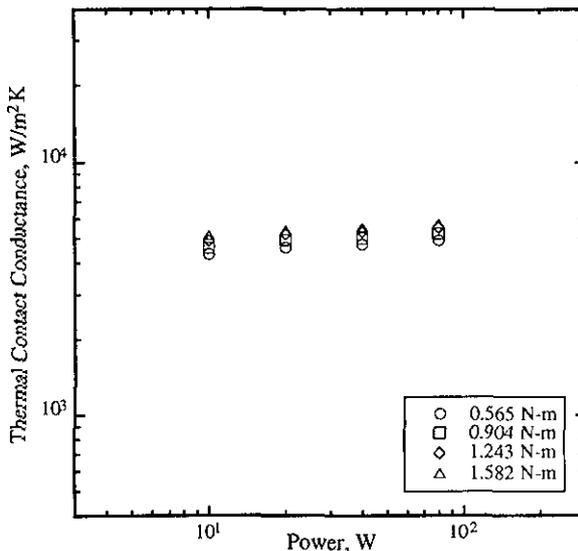
Figure 5 Thermal contact conductance as a function of module power dissipation for Type III anodized SEM-E frame guide rib to Type II anodized chassis card rail.
