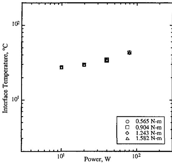
Figure 9 Interface temperature as a function of module power dissipation for Type III anodized SEM-E frame guide rib to Type II anodized chassis card rail.
