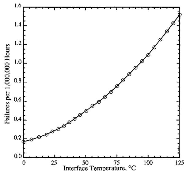
Figure 1 Influence of interface temperature on device failure (per 1000000 Hours), from Beasley<sup>2</sup>.
