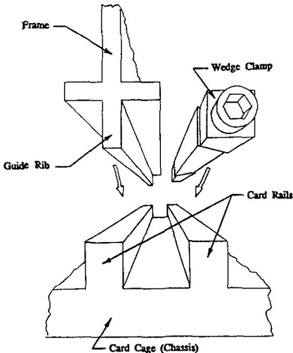
Figure 2 Exploded view of Standard Electronic Module (SEM) junction.
