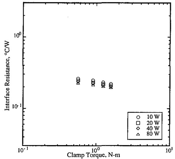
Figure 8 Interface resistance as a function of clamp torque for Type III anodized SEM-E frame guide rib to Type II anodized chassis card rail.
