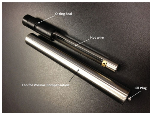
Fig. 2—Hot-wire probe to be inserted into the volume compensation can.
