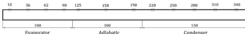
Fig. 2. Thermocouple position of heat pipe.
