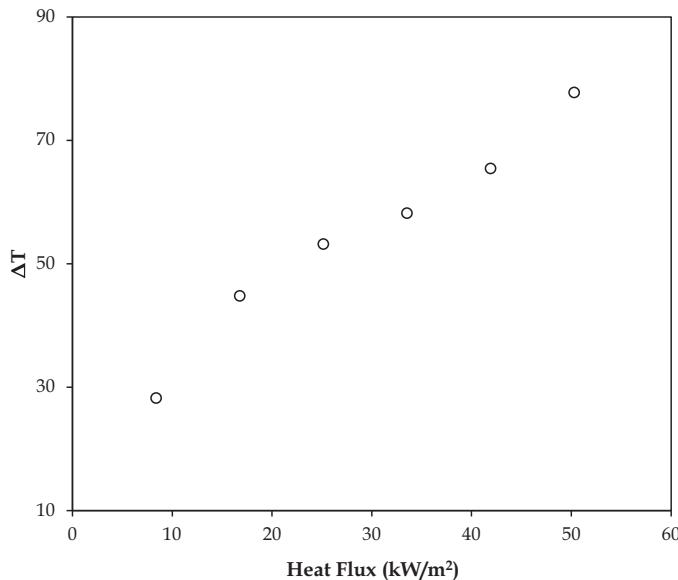
Fig. 5. Temperature difference of heat pipe at different heat fluxes.
