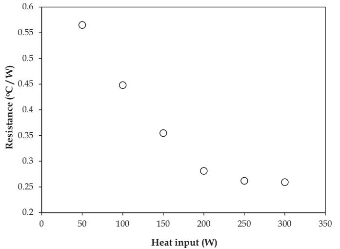
Fig. 6. Thermal resistance of heat pipe at different heat inputs.
