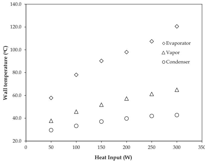
Fig. 4. Temperature responses of heat pipe at different heat inputs.
