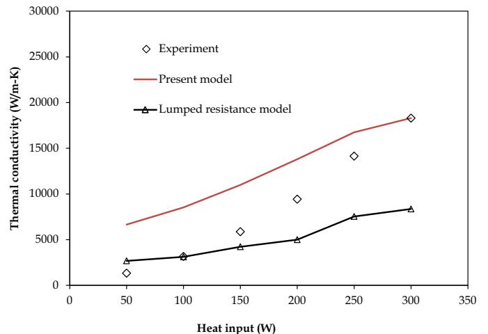
Fig. 7. Thermal conductivity of heat pipe at different heat inputs.
