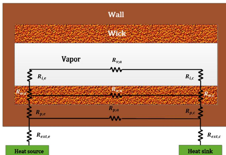
Fig. 3. Lumped thermal resistance network.
