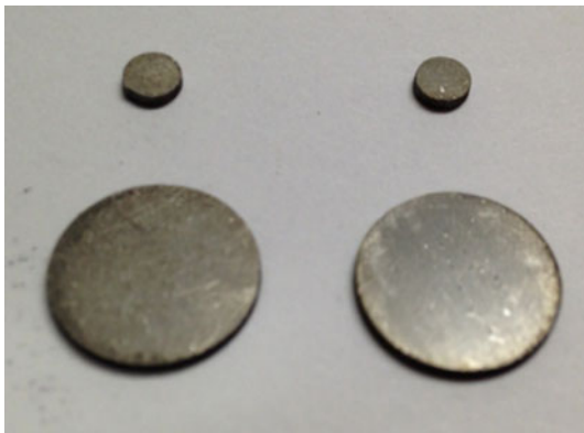
Fig. 2. Round-robin 1 samples sent to each laboratory: two p -type (left) and two n -type (right) samples.
