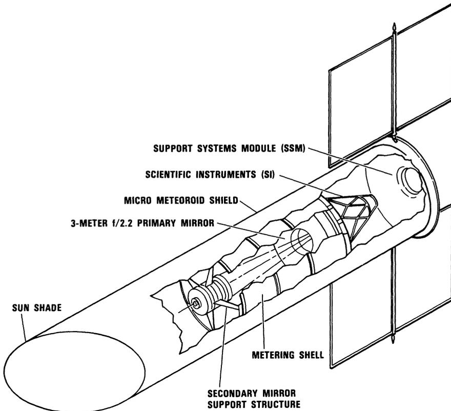
*Figure 1. The Space Telescope (Phase A version).*
