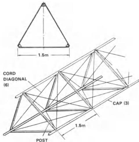
Figure 11. Beams employ lightweight, open-truss construction.
