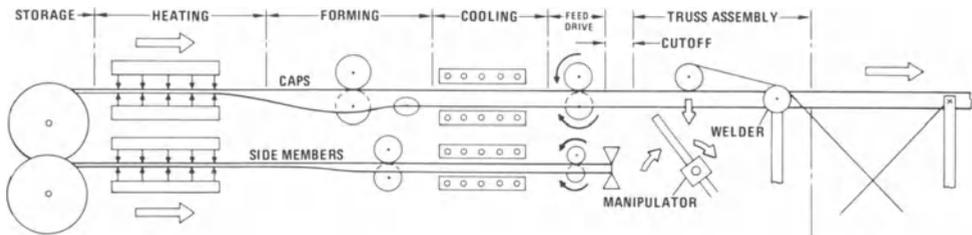
*Figure 12. Semi-schematic of the beam builder (typical for three places).*
