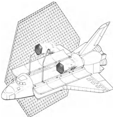
Figure 10. Deployable structure modules in the Shuttle.
