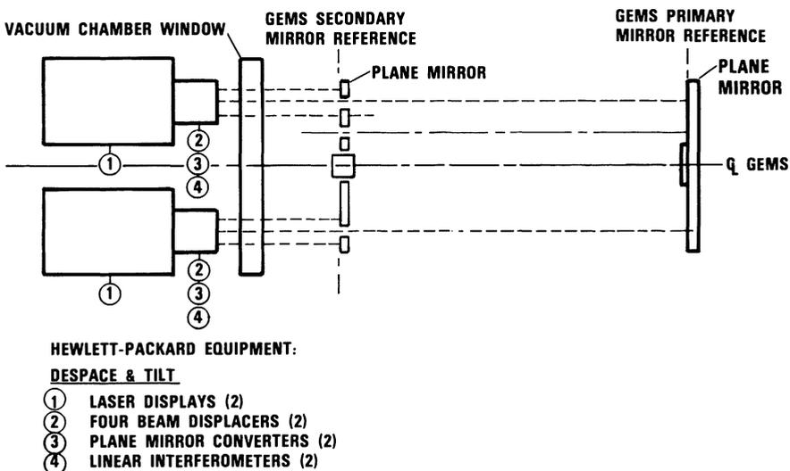
Figure 3. The Laser Dilatometer.
