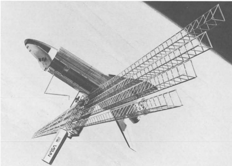
*Figure 13. A single Space Shuttle mission fabricates and assembles a 200-meter long platform.*
