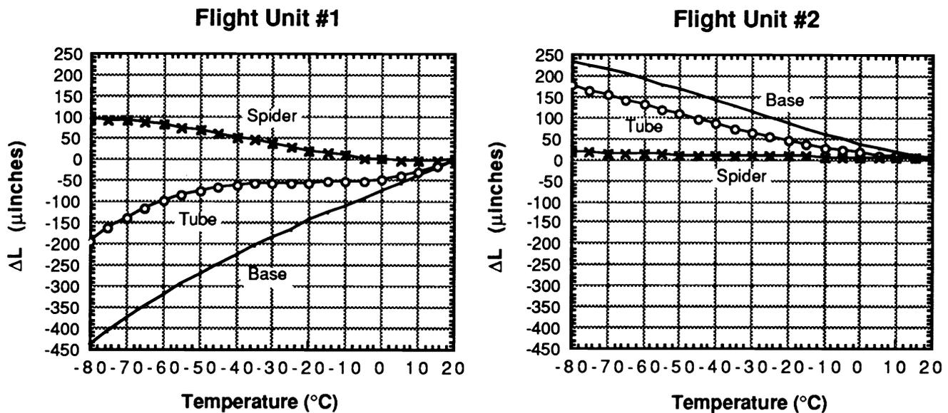
Figure 4.3. Relative displacements between the primary and secondary mirror mounting surfaces of the Flight Unit #1 (a) and Flight Unit #2 (b) graphite/epoxy structures.
