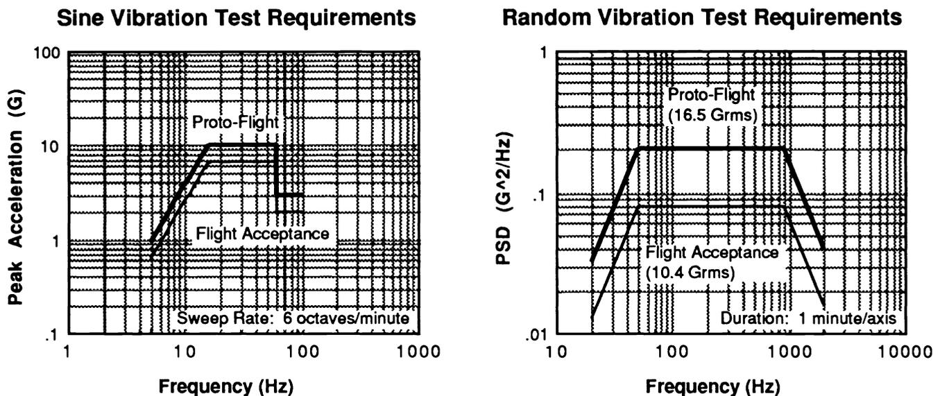
Figure 3.1. Sine vibration test requirements (a) and random vibration test requirements (b) for Mars Observer Spacecraft nadir panel-mounted instruments.
