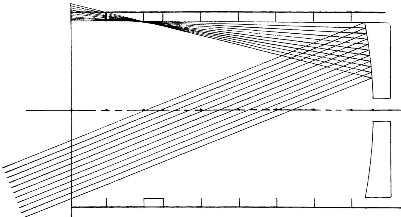
Figure 2.1. Concentration of solar radiation on the spider stiffening annulus at  $22^\circ$  from axis.
