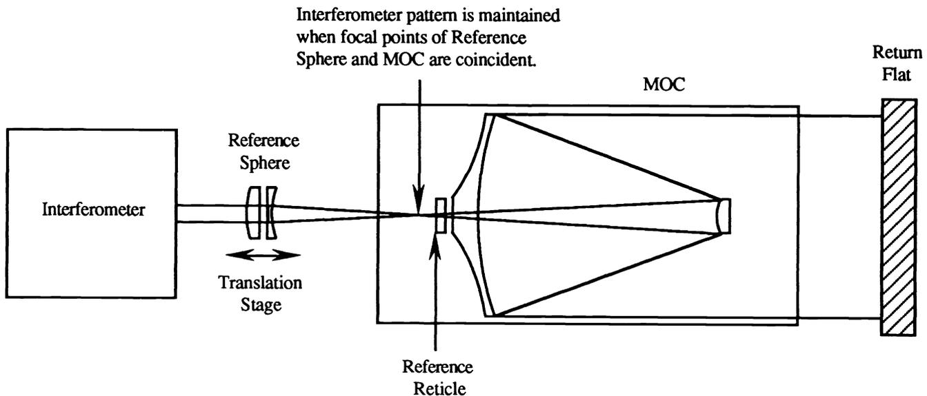
Figure 5.1. MOC interferometric test set up. MOC axial focal point displacements can be measured directly by the reference sphere displacement required to regain the interferometric pattern.
