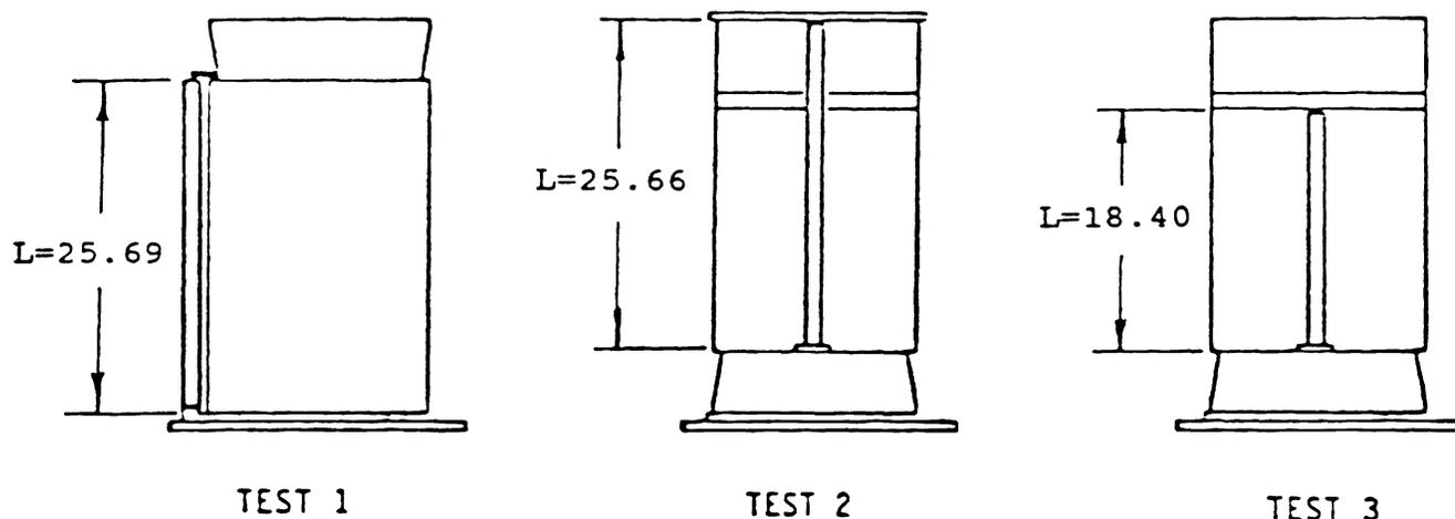
Figure 4.2. Test configurations to derive the  $\Delta L(T)$  of the tube (a), the base (b), and the spider (c).
