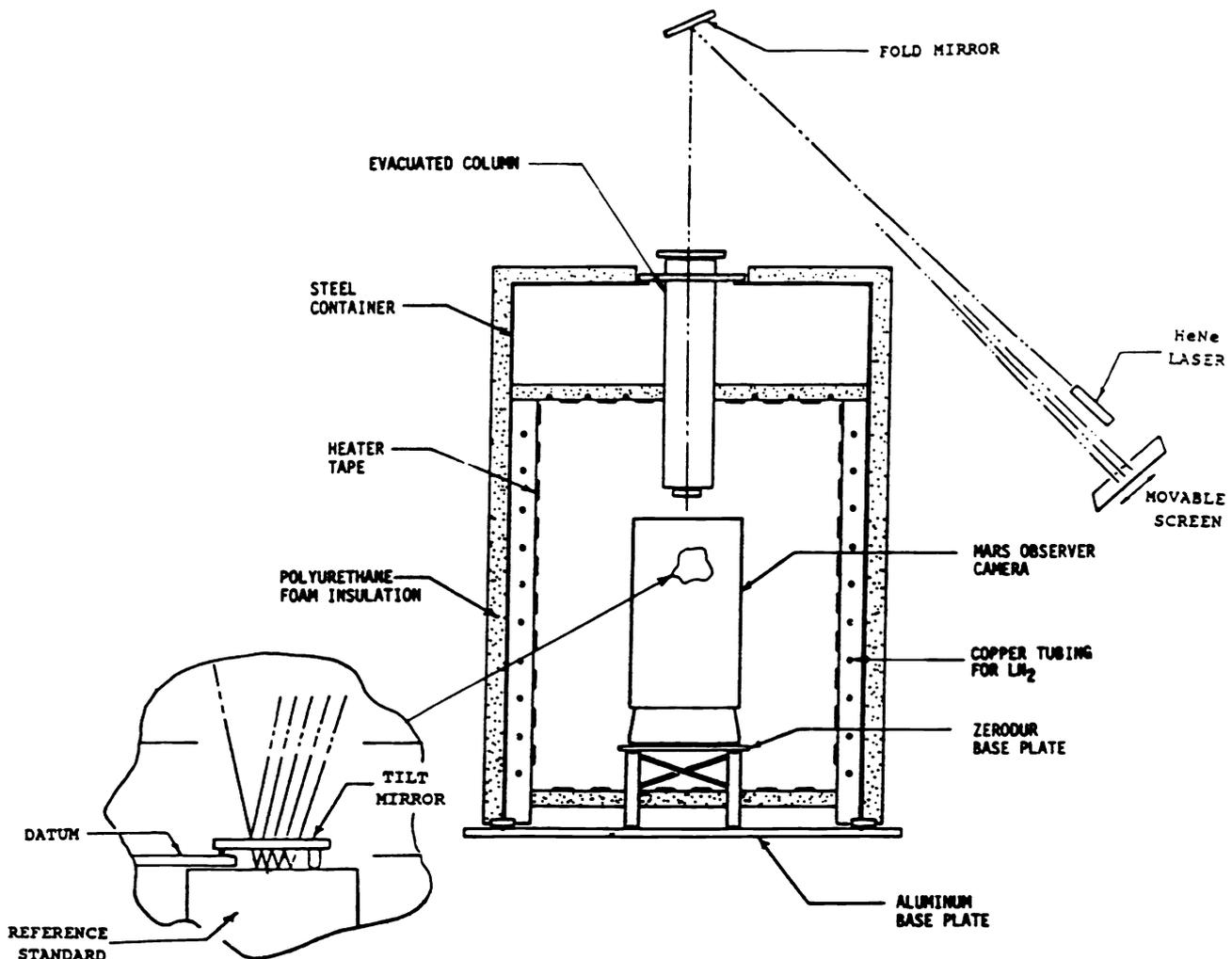
Figure 4.1. COI thermal expansion dilatometer set-up.
