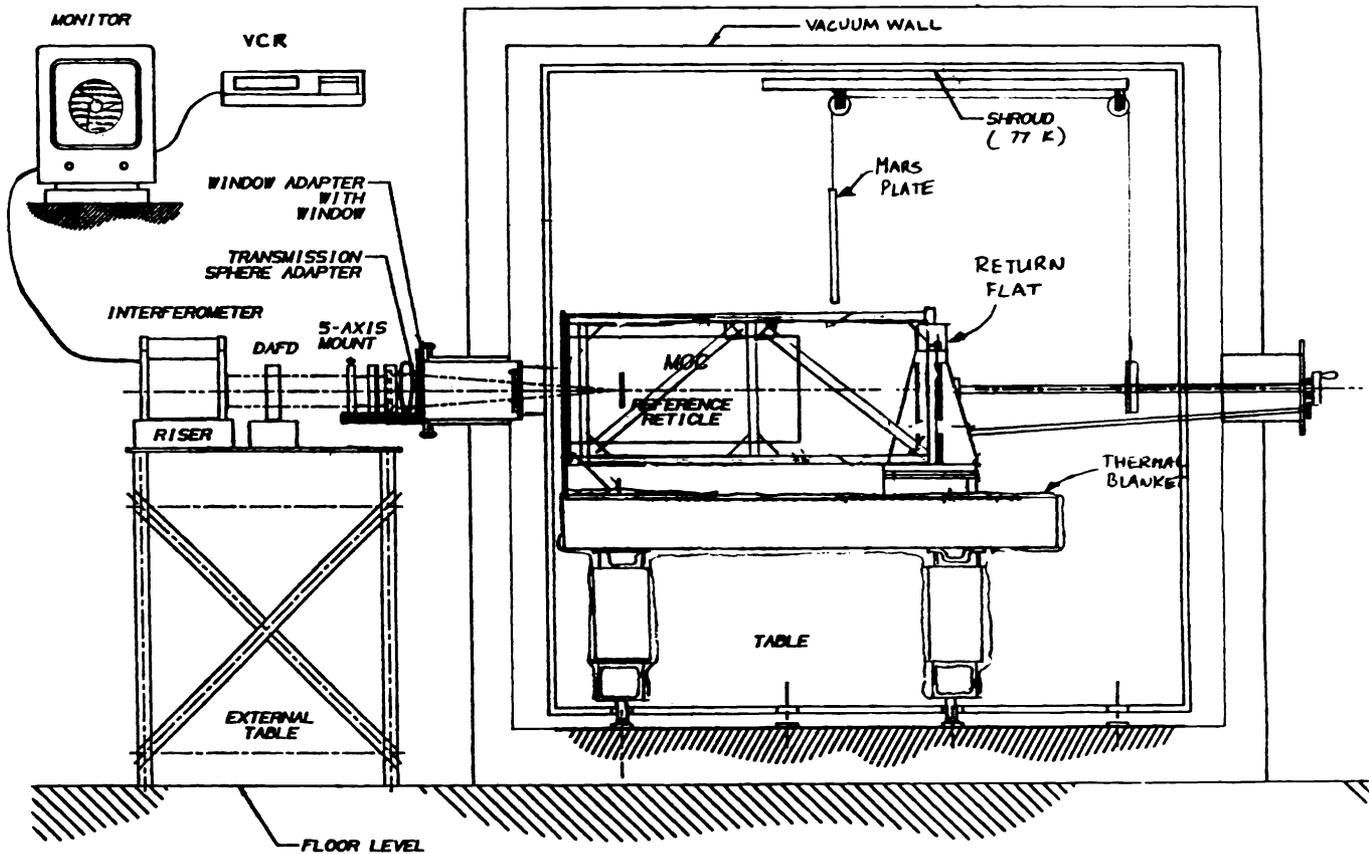
Figure 5.2. MOC thermal-vac test set-up.
