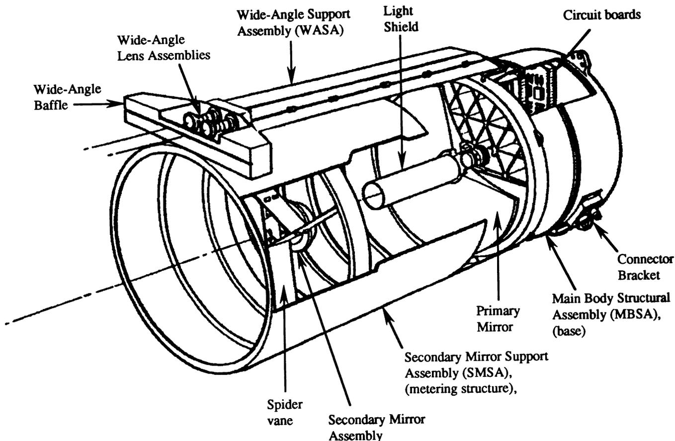
Figure 1. MOC Flight Unit cutaway view.
