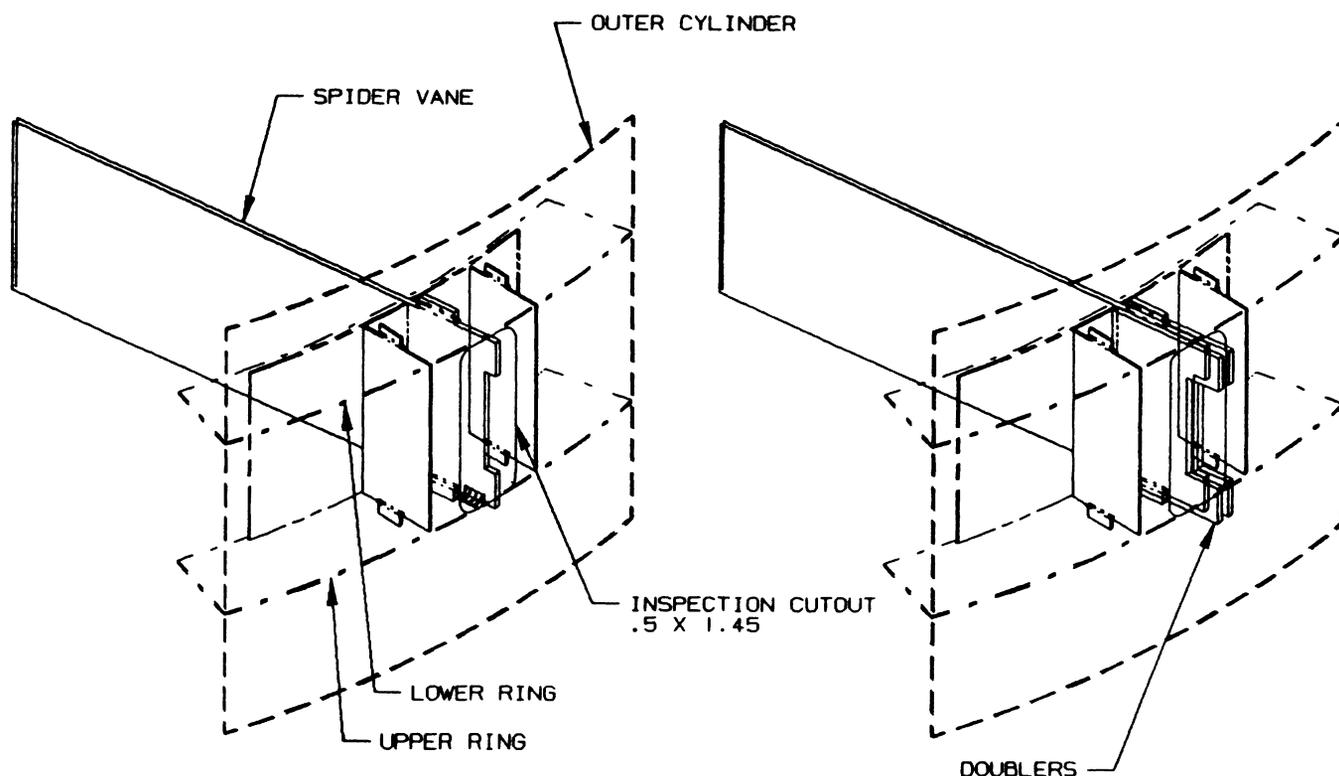
Figure 3.2. Spider stiffening annulus inspection and repair.
