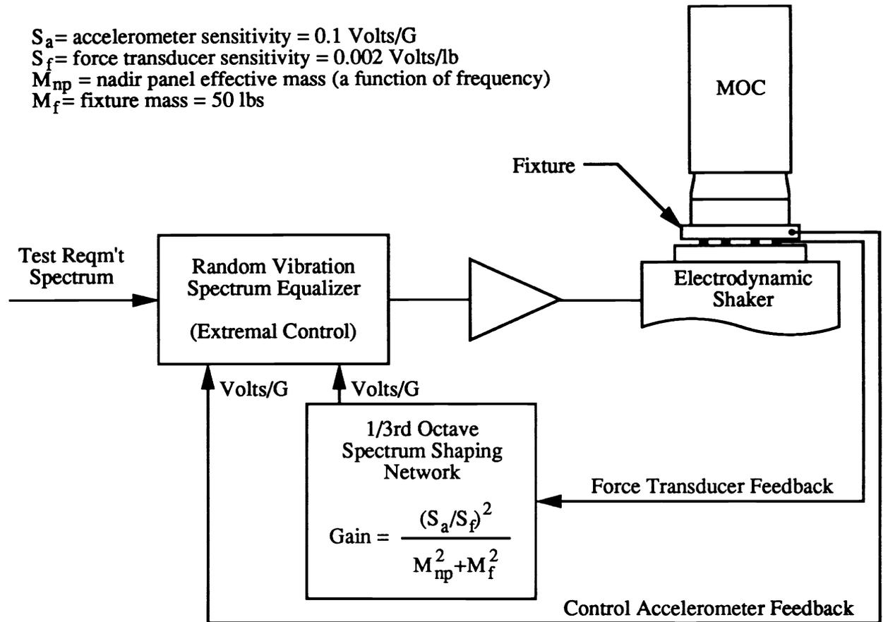
Figure 3.3. Force limiting control loop.
