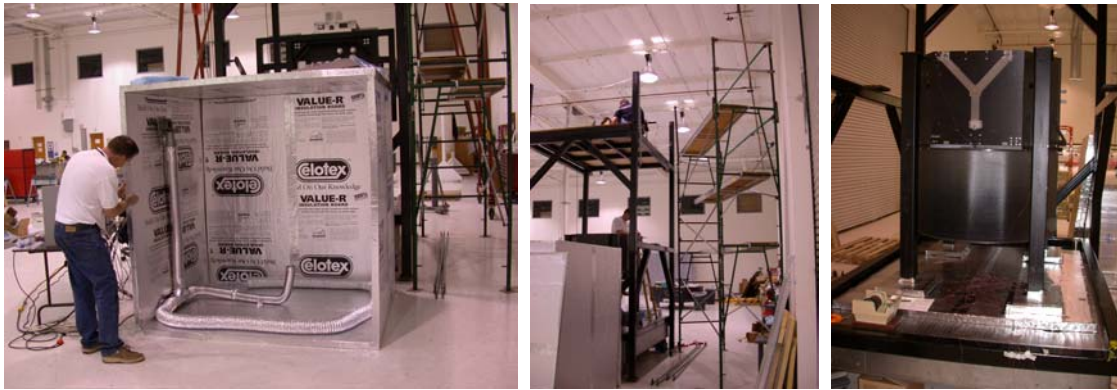
Figure 4: Thermal Chamber Test Run (left), Support Tower (middle), Structure During Test Integration (right)
