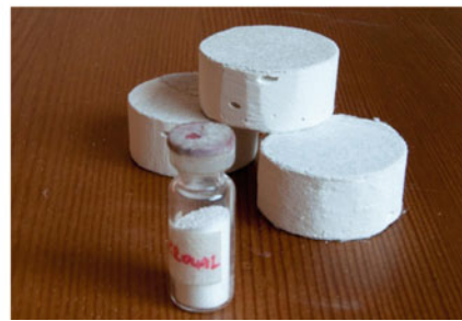
Fig. 3 Structure of microcapsules with phase change wax of Micronal ® PCM [5] and real specimen (microcapsules of Micronal ® PCM in gypsum)
