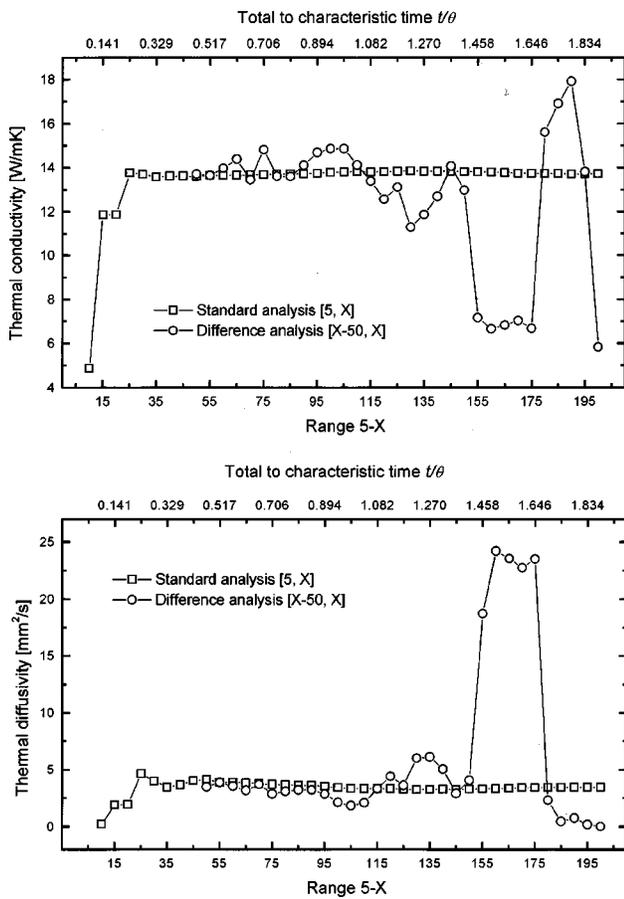
FIG. 4. The plot of thermal conductivity and thermal diffusivity as a function of time used in the fitting procedure for stainless steel. The standard and differential analyses show good agreement with predictions by the theoretical sensitivity coefficients.
