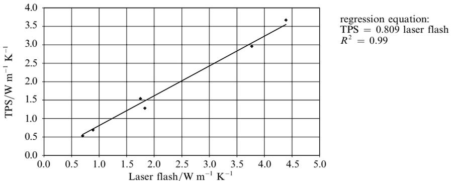
**Figure 7.** Thermal conductivity results from the two techniques show a linear relationship but with a 20% bias.
