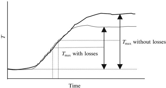
**Figure 8.** Heat losses at the surfaces shifts the penetration time to a lower value, indicating a higher diffusivity.
