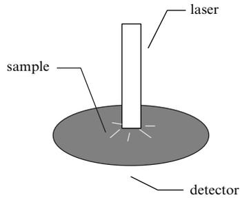
**Figure 3.** Experimental diagram for laser flash diffusivity testing.
