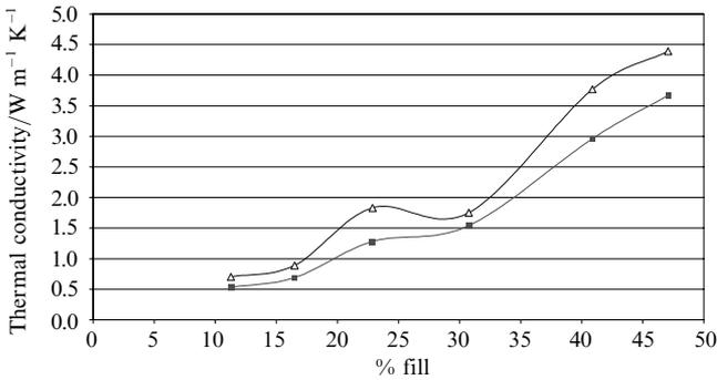
**Figure 6.** Thermal conductivity increased with percent fill of alumina:  $\Delta$ , laser flash method;  $\blacksquare$ , TPS method.
