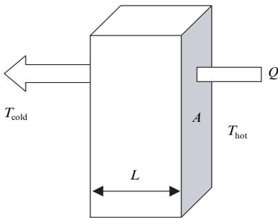
**Figure 1.** Experimental variables for steady state thermal conductivity tests.
