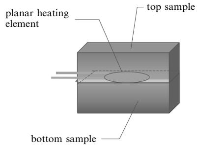
**Figure 5.** Experimental setup for transient plane source testing.
