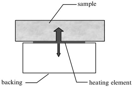
**Figure 4.** Experimental setup for the modified hot wire technique.
