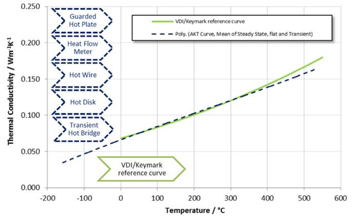
Fig. 9. Comparison of VDI/Keymark reference curve (dashed curve) with the AKT Curve, mean polynomial of the measured values of the steady state, flat, and transient methods (solid line) as a function of temperature.
