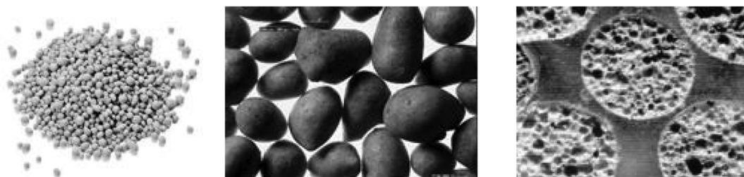
**Fig. 1.** Investigated expanded glass granulate Liaver<sup>®</sup>: loose bed (left), single granules with a granule size of approximately 1 mm–2 mm (middle) and cross sections through single granules (right).
