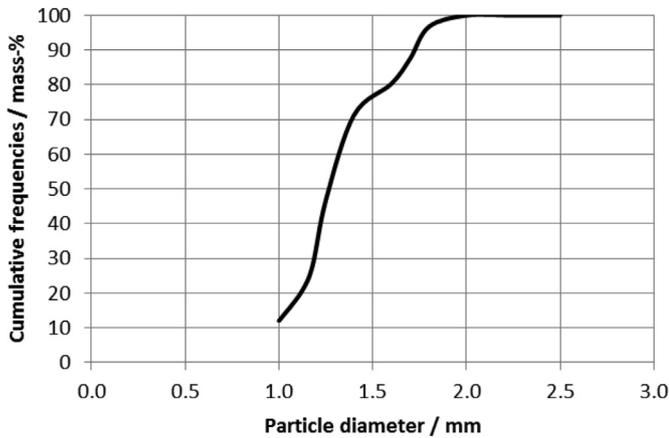
Fig. 2. Distribution of cumulative frequencies of particle diameter of the investigated expanded glass granulate Liaver®.
