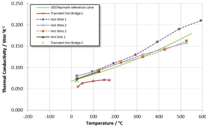
Fig. 7. All measured thermal conductivity values of the transient method and the VDI/Keymark reference curve as a function of temperature.
