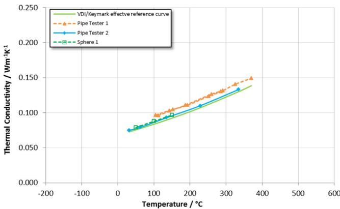
Fig. 8. Measured values of the steady state method for "other" apparatus and the VDI/Keymark effective reference curve as a function of temperature at higher temperature differences.
