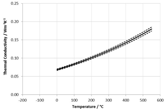
Fig. 4. Thermal conductivity VDI/Keymark reference curve of the investigated expanded glass granulate Liaver<sup>®</sup> as a function of temperature (solid line) with the uncertainty criteria of  $\pm 3\%$  (dashed lines).
