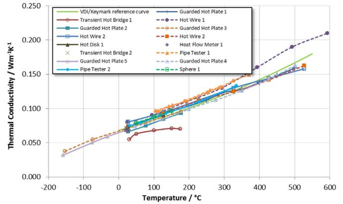
Fig. 5. Experimentally determined thermal conductivity values of all participants and the VDI/Keymark reference curve as a function of temperature.
