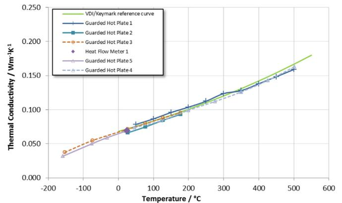
Fig. 6. All measured values of the steady state method for flat specimens, and the VDI/Keymark reference curve as a function of temperature.
