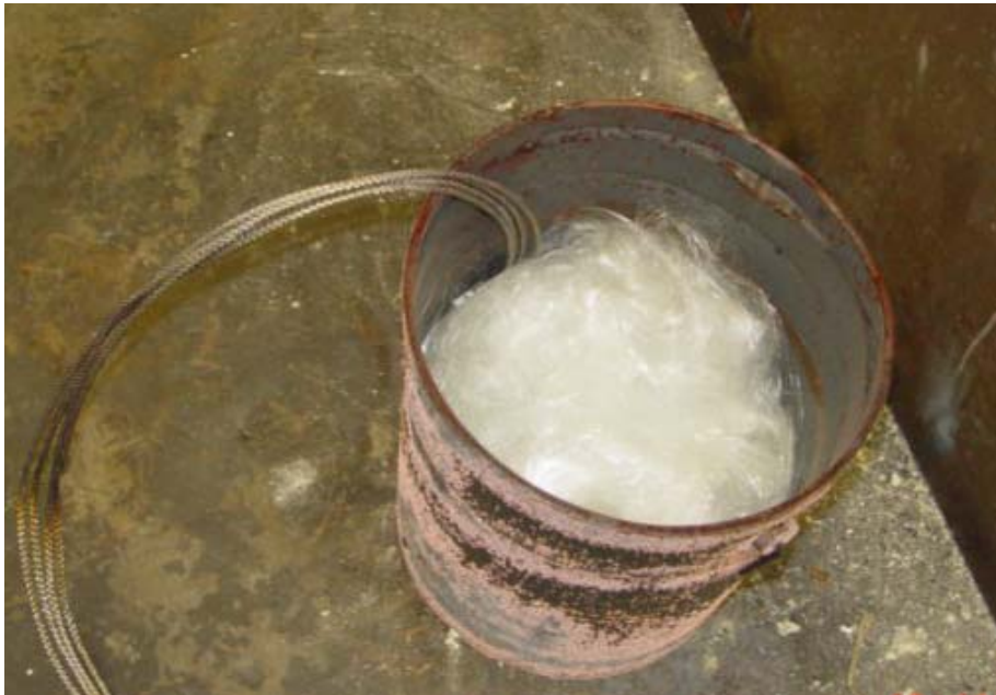
Figure 3. The glass fibers are packed inside a bucket. The Hot Disk sensor is placed in the middle of the sample using shielded high temperature wire.
