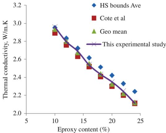
**Figure 7.** Comparison of effective thermal conductivity.
