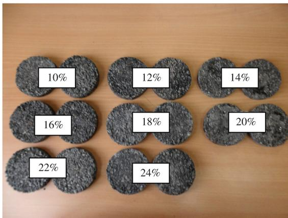
**Figure 1.** Test specimens with varying epoxy content.
