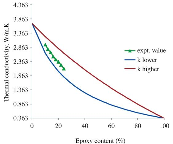
Figure 6. H-S bound chart for epoxy granite material.
