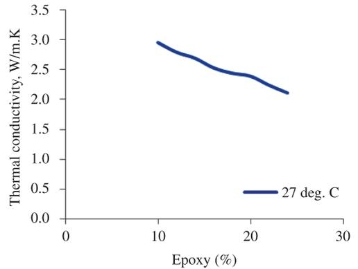
Figure 5. Variation of effective thermal conductivity with variation in epoxy content.
