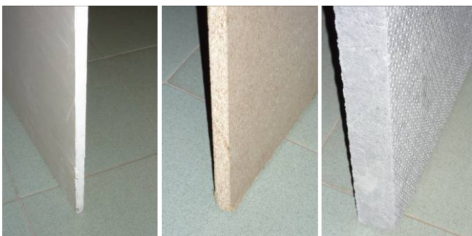
Figure 8. Pictures of the analyzed samples: plasterboard, plywood, and expanded polystyrene.
