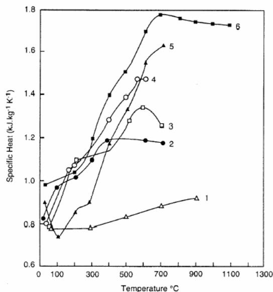
**Figure 6.** Effect of temperature on measured specific heat of various concretes. Compilation made by Bažant and Kaplan (1996). (1) granite aggregate concrete (Ödeen, 1968); (2) limestone aggregate concrete (Collet and Tavernier, 1976); (3) lime stone aggregate concrete (Harmathy and Allen, 1973); (4) siliceous aggregate concrete (Harmathy and Allen, 1973); (5) limestone aggregate concrete (Hildebrand, et al., 1978); (6) siliceous aggregate concrete (Hildebrand, et al., 1978)
