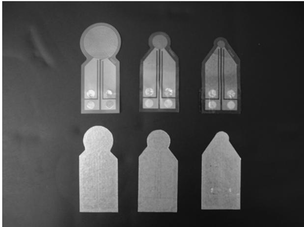
**Figure 13.** The upper three sensors are insulated with Kapton and the lower three with Mica.
