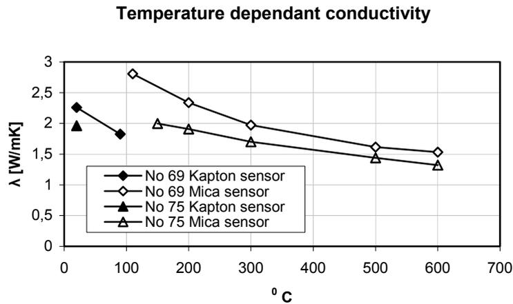
**Figure 39.** The temperature dependent thermal conductivity for self-compacting concrete. The discrepancy in conductivity for test specimen no 69 is when the sensor was switched from a radius 9.719 mm Kapton to a radius 6.631 mm Mica.
