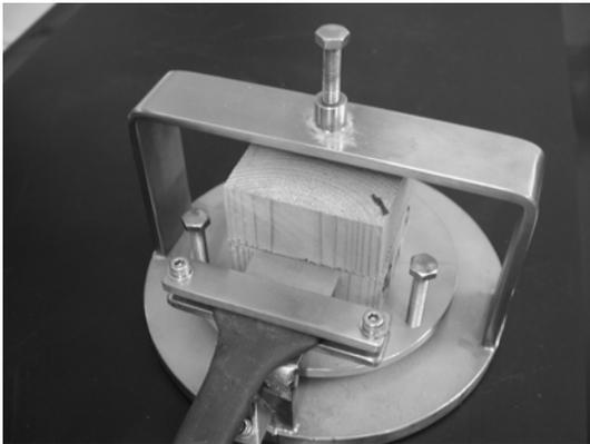
**Figure 21.** The test setup with a wood test specimen and sample holder for a measurement at room temperature.
