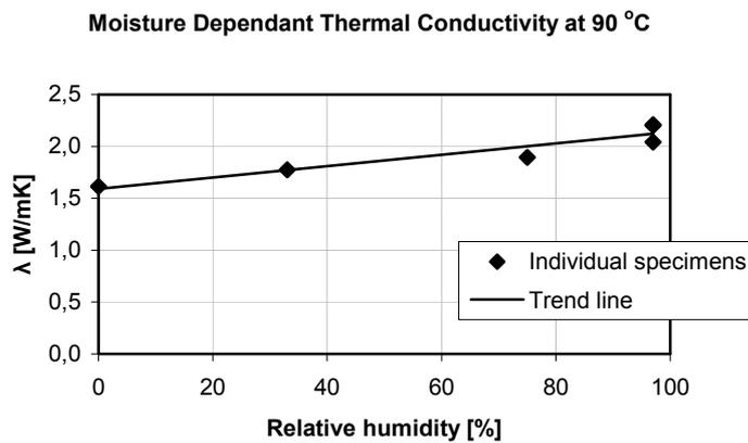
**Figure 28.** The moisture dependent thermal conductivity for conventional concrete at 90 °C. The relative humidity on the x –axis is at room temperature prior the testing.
