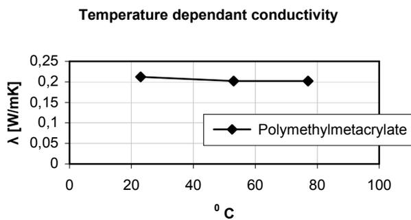
**Figure 56.** The temperature dependent thermal conductivity for polymethylmetacrylate.
