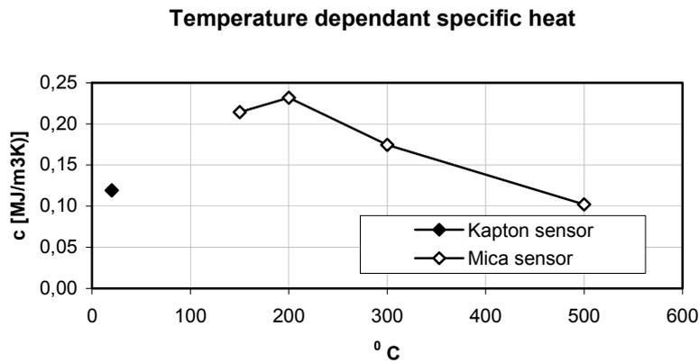
**Figure 61.** The temperature dependent specific heat for glass wool.
