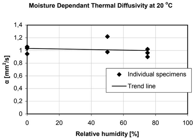
**Figure 37.** The moisture dependent thermal diffusivity for high performance concrete at 20 °C. The trend line in the diagram is a coarse assumption but it may give an indication of the difference.
