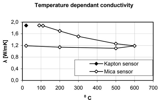
**Figure 69.** The thermal conductivity for the tested concrete at different temperatures and place in the heating cycle. The heating cycle starts at the highest conductivity value at 20 °C.
