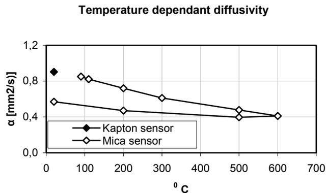
**Figure 70.** The thermal diffusivity for the tested concrete at different temperatures and place in the heating cycle. The heating cycle starts at the highest diffusivity value at 20 °C.
