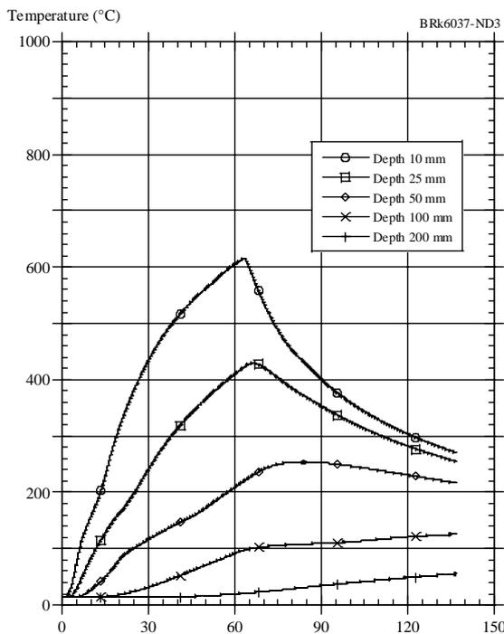
**Figure 68.** Measured temperatures at different depths of the test specimen (Boström 2004).
