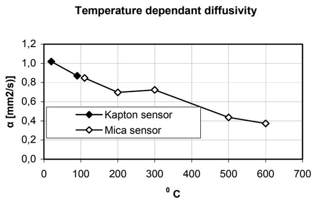
**Figure 34.** The temperature dependent thermal diffusivity for high performance concrete.
