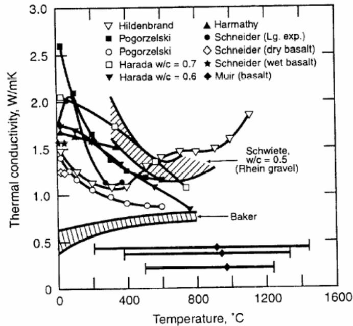
**Figure 5.** Thermal conductivity of siliceous-aggregate concrete. Compilation made by Schneider (1982).
