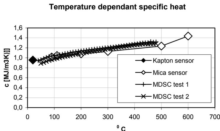
**Figure 71.** Specific heat measured with the TPS method and a Modulated Differential Scanning Calorimeter.
