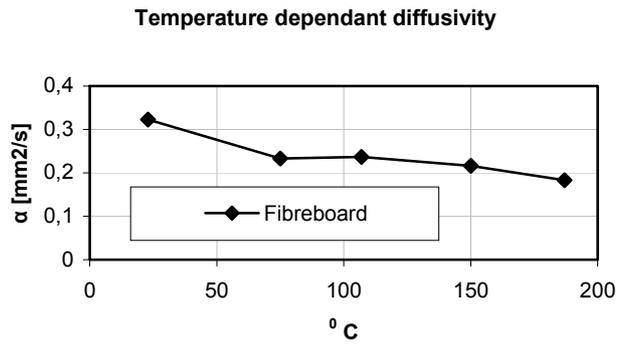
**Figure 54.** The temperature dependent thermal diffusivity for fibreboard.
