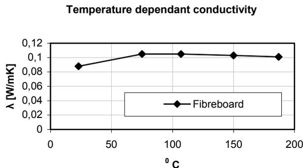
**Figure 53.** The temperature dependent thermal conductivity for fibreboard.
