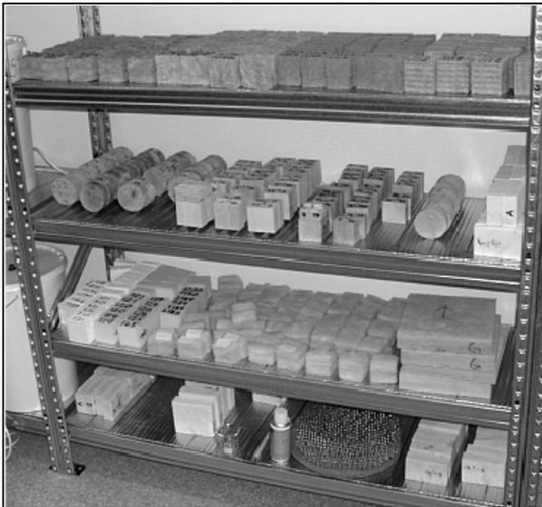
**Figure 16.** Test specimens stored in a climate room.
