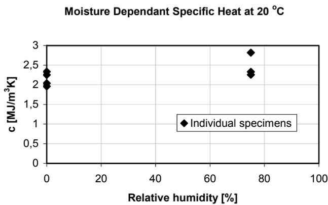
**Figure 44.** The moisture dependent specific heat for self-compacting concrete at 20 °C.
