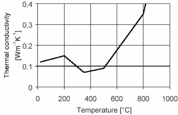
**Figure 9.** Thermal conductivity for wood and char layer according to Eurocode 5: Part 1-2 (2003).
