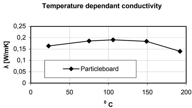
**Figure 50.** The temperature dependent thermal conductivity for particleboard.
