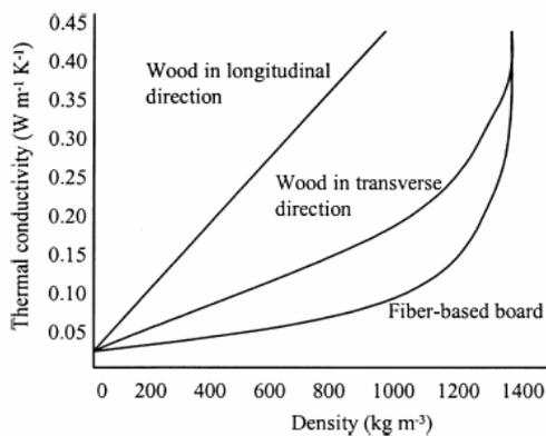
**Figure 8.** Effect of density on thermal conductivity of wood and fibre-based board at 12 % moisture content and temperature 300 K (Kollman and Cote 1968).
