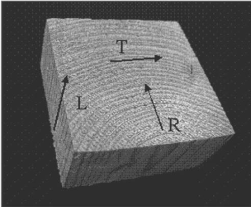
**Figure 7.** Principle directions in wood: R = Radial, T =Tangential and L =Longitudinal
