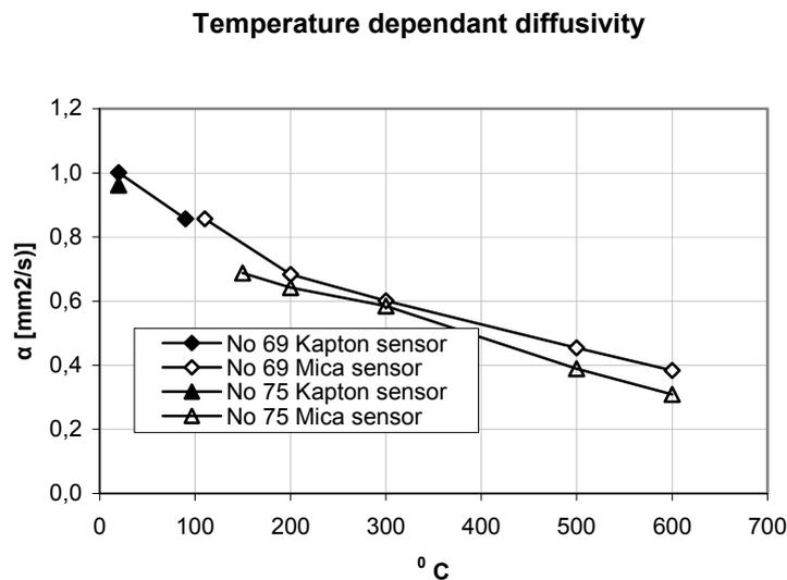
**Figure 40.** The temperature dependent thermal diffusivity for self-compacting concrete.
