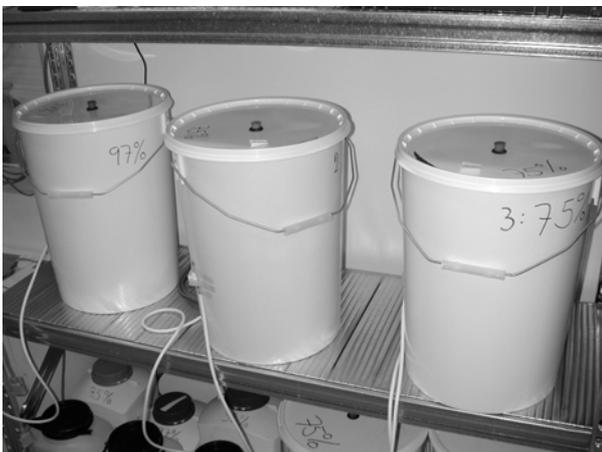
**Figure 17.** Buckets with salt solutions in which specimens were stored.
