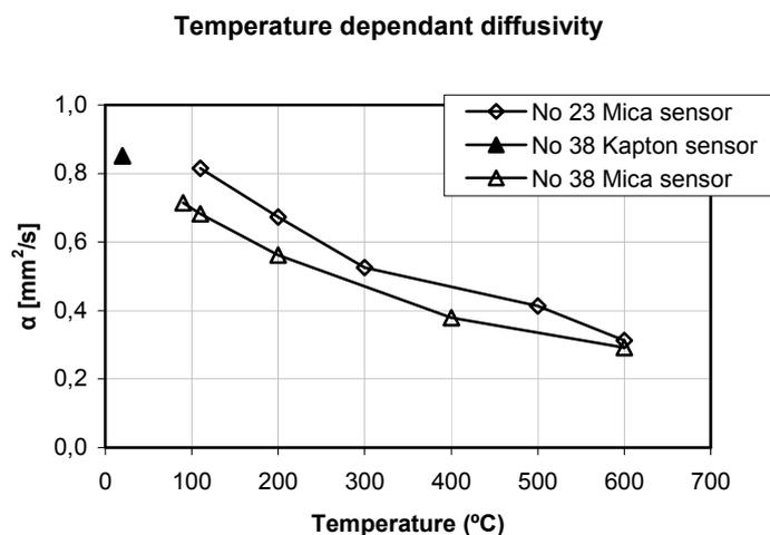
**Figure 24.** The temperature dependant thermal diffusivity for conventional concrete.
