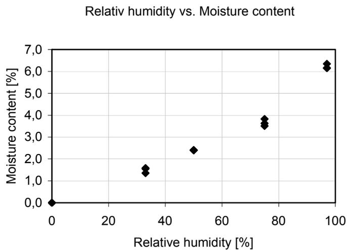
**Figure 26.** The relation between relative humidity and moisture content for the conventional concrete specimens.
