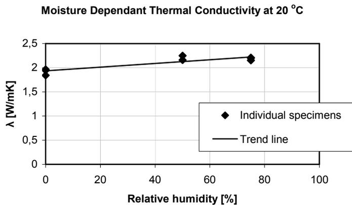
**Figure 36.** The moisture dependent thermal conductivity for high performance concrete at 20 °C. The trend line in the diagram is a coarse assumption but it may give an indication of the difference.
