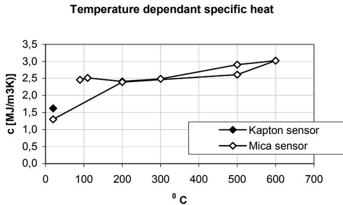
**Figure 47.** The temperature dependent specific heat for cement paste. The diagram also includes measurements from the cooling down (the lower values).
