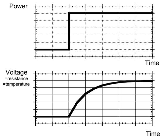
**Figure 12.** When the stepwise power pulse is applied the change in voltage is recorded and converted to resistance and thereafter temperature.
