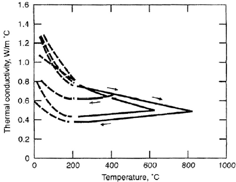
**Figure 1.** Temperature dependent thermal conductivity for concrete with  $w/c = 0.7$  (Ödeen and Nordström 1972). The cooling phase is included in the diagram.
