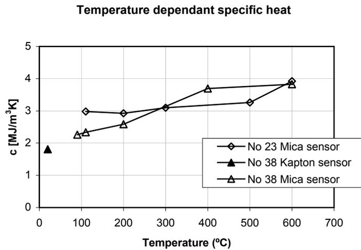
**Figure 25.** The temperature dependent specific heat for conventional concrete.
