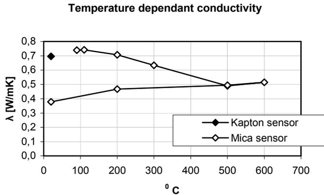
**Figure 45.** The temperature dependent thermal conductivity for cement paste. The diagram also includes measurements from the cooling down (the lower values). Switched from a radius 9.719 mm Kapton to a radius 6.631 mm Mica at 90 °C.
