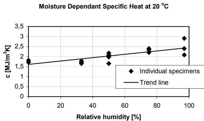
**Figure 31.** The moisture dependent specific heat for conventional concrete at 20 °C.
