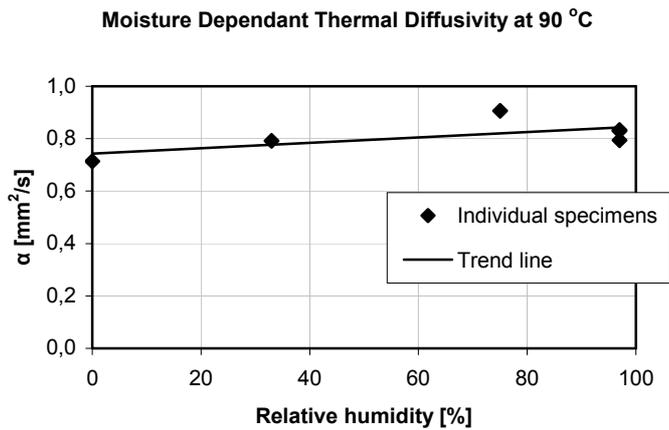
**Figure 30.** The moisture dependent thermal diffusivity for conventional concrete at 90 °C. The relative humidity on the x –axis is at room temperature prior the testing.
