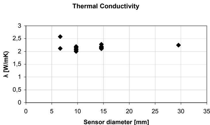
**Figure 22.** The diagram shows measurements on the same test specimen with different sensors and positions.
