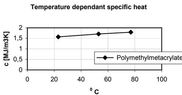
**Figure 58.** The temperature dependent specific heat for polymethylmetacrylate.
