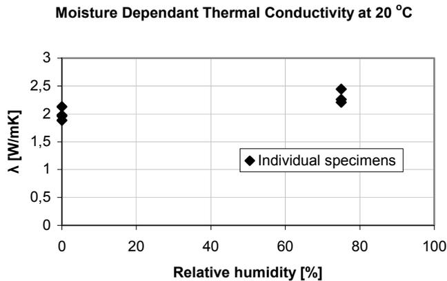
**Figure 42.** The moisture dependent thermal conductivity for self-compacting concrete at 20 °C.
