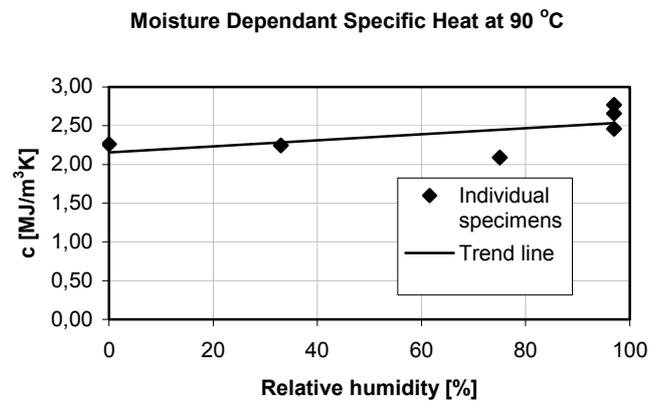
**Figure 32.** The moisture dependent specific heat for conventional concrete at 90 °C. The relative humidity on the x –axis is at room temperature prior the testing.
