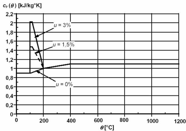
**Figure 4.** Specific heat for siliceous concrete as a function of temperature at three different moisture contents according to Eurocode 2 part 1-2 (2003).
