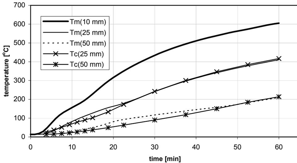
**Figure 72.** Temperature curves from the measurement, Tm = temperature measurement, Tc = temperature calculation.
