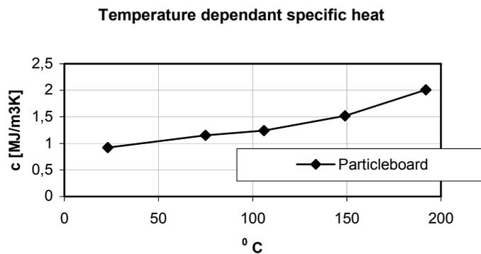
**Figure 52.** The temperature dependent specific heat for particleboard.
