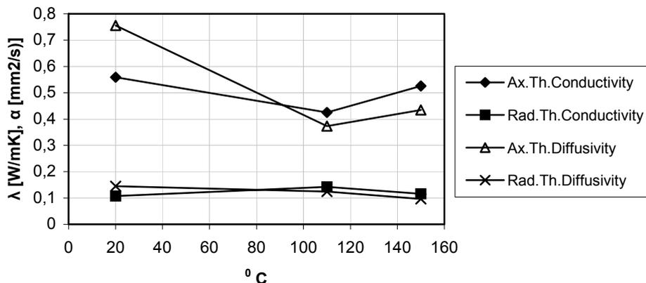
**Figure 48.** The temperature dependent axial and radial thermal conductivity and diffusivity for high-density spruce. Axial in the measurements is longitudinal in the material and radial is radial and tangential in the living tree.
