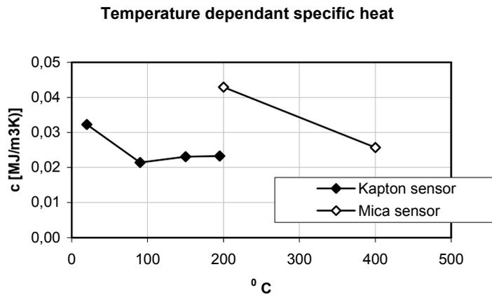
**Figure 64.** The temperature dependent specific heat for low-density glass wool. There is an unphysical jump between the different sensors, see previous chapter.
