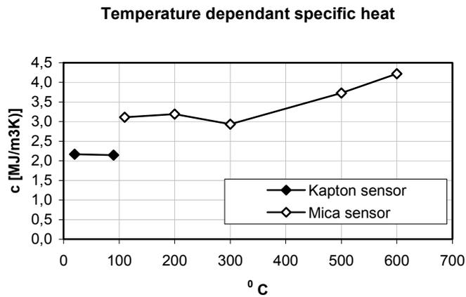
**Figure 35.** The temperature dependent specific heat for high performance concrete. The discrepancy in specific heat is when the sensor was switched from a radius 9.719 mm Kapton to a radius 6.631 mm Mica.
