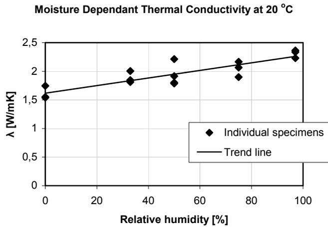
**Figure 27.** The moisture dependent thermal conductivity for conventional concrete at 20 °C. Test specimens conditioned at different relative humidity.
