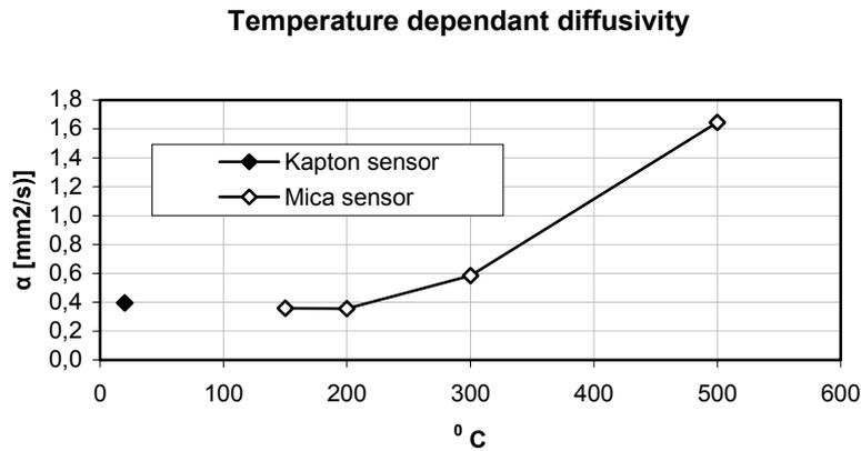
**Figure 60.** The temperature dependent thermal diffusivity for glass wool.
