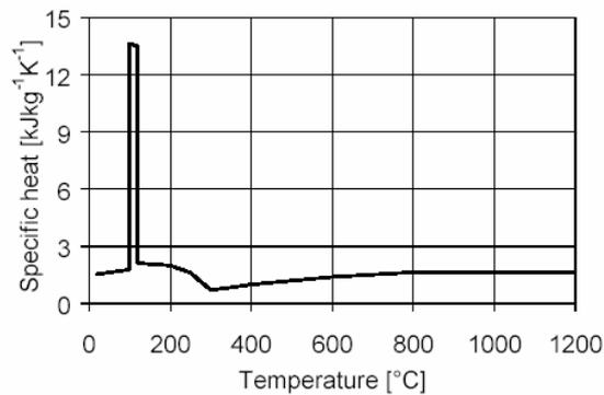
**Figure 10.** Specific heat for wood and charcoal according to Eurocode 5: Part 1-2 (2003). The peak in the diagram is the latent heat of evaporation.
