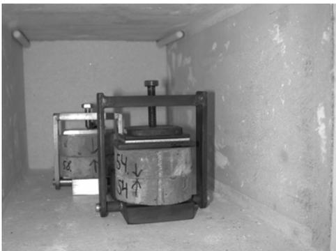
**Figure 20.** Two test specimens placed inside a test furnace.
