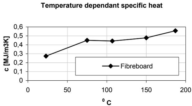
**Figure 55.** The temperature dependent specific heat for fibreboard.
