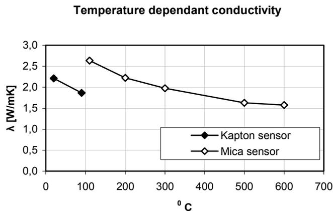
**Figure 33.** The temperature dependent thermal conductivity for high performance concrete. The discrepancy in conductivity is when the sensor was switched from a radius 9.719 mm Kapton to a radius 6.631 mm Mica. The test specimen was dried before the test.
