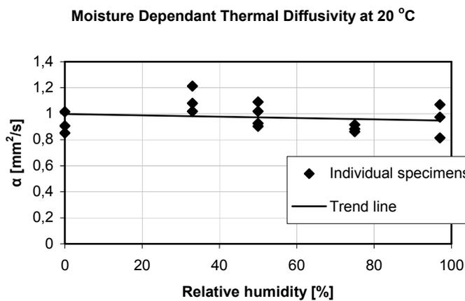
**Figure 29.** The moisture dependent thermal diffusivity for conventional concrete at 20 °C.
