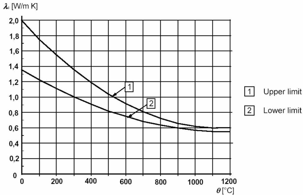
**Figure 3.** Thermal conductivity of concrete according to Eurocode 2 part 1-2 (2003).
