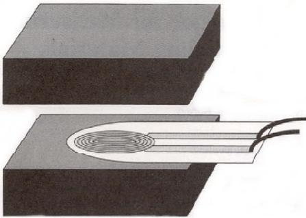
**Figure 11.** Test setup for a measurement according to the TPS method (Gustafsson and Long 1995).
