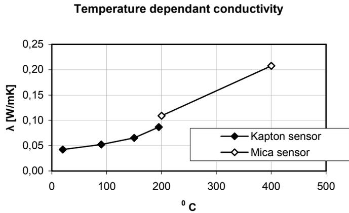
**Figure 62.** The temperature dependent thermal conductivity for low-density glass wool. There is an unphysical jump between the different sensors, see previous chapter.
