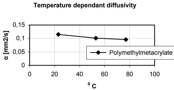
**Figure 57.** The temperature dependent thermal diffusivity for polymethylmetacrylate.
