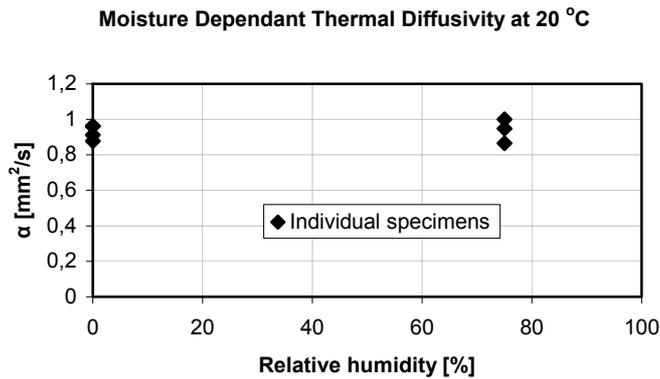
**Figure 43.** The moisture dependent thermal diffusivity for self-compacting concrete at 20 °C.
