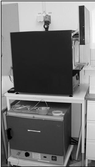
**Figure 19.** Ovens used for heating the specimens.
