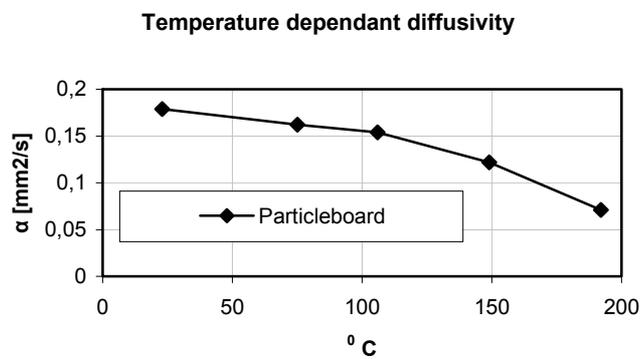
**Figure 51.** The temperature dependent thermal diffusivity for particleboard.
