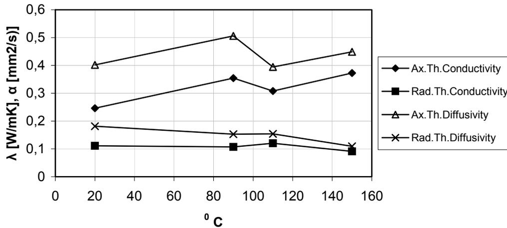
**Figure 49.** The temperature dependent axial and radial thermal conductivity and diffusivity for low-density spruce. Axial in the measurements is longitudinal in the material and radial is radial and tangential in the living tree.
