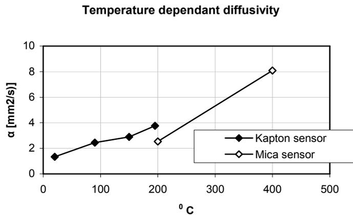
**Figure 63.** The temperature dependent thermal diffusivity for low-density glass wool. There is an unphysical jump between the different sensors, see previous chapter.
