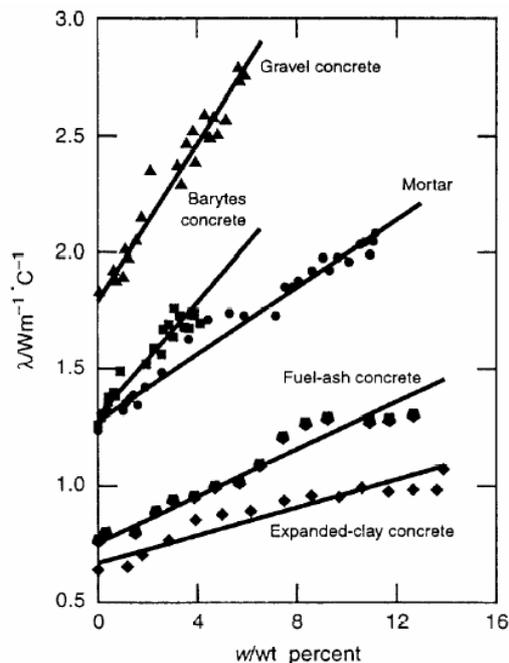
**Figure 2.** Thermal conductivity versus moisture content of different kind for concrete (Morabito 1989).
