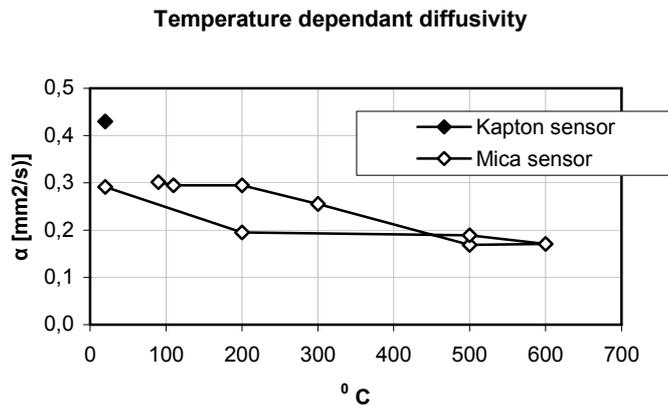
**Figure 46.** The temperature dependent thermal diffusivity for cement paste. The diagram also includes measurements from the cooling down (the lower values).
