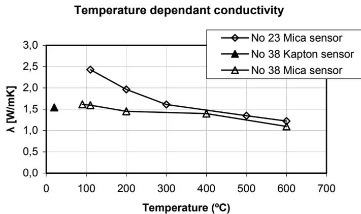
**Figure 23.** The temperature dependent thermal conductivity for conventional concrete. The sensor radius was 9.719 mm for both the used Kapton and Mica sensors. Specimen No 23 were in equilibrium with 33% RH prior test and No 38 was dried before the test.
