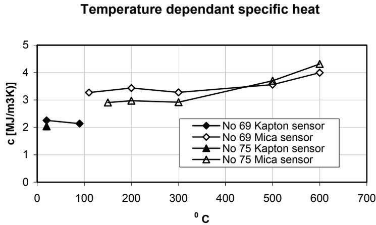
**Figure 41.** The temperature dependent specific heat for self-compacting concrete. The discrepancy in specific heat for test specimen no 69 is when the sensor was switched from a radius 9.719 mm Kapton to a radius 6.631 mm Mica.
