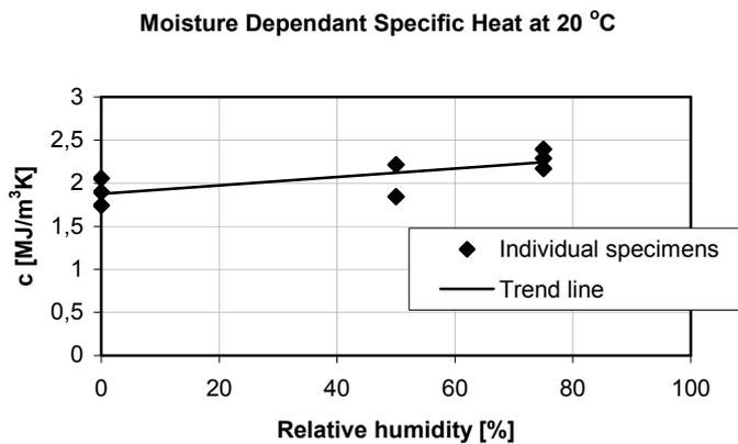
**Figure 38.** The moisture dependent specific heat for high performance concrete at 20 °C. The trend line in the diagram is a coarse assumption but it may give an indication of the difference.
