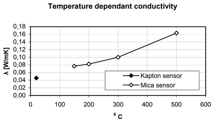
**Figure 59.** The temperature dependent thermal conductivity for high-density glass wool.
