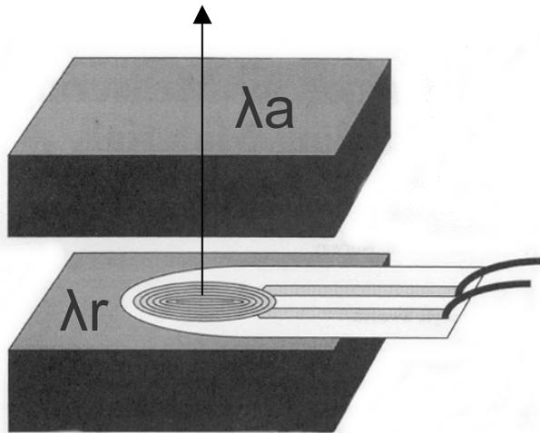
**Figure 14.** The radial and axial directions in the anisotropic solution in the material in comparison with the sensor position.
