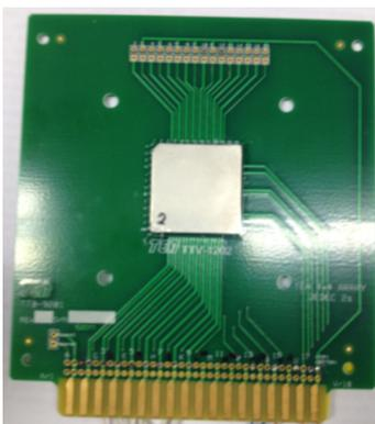
Figure 2. The top view of the real test vehicle
