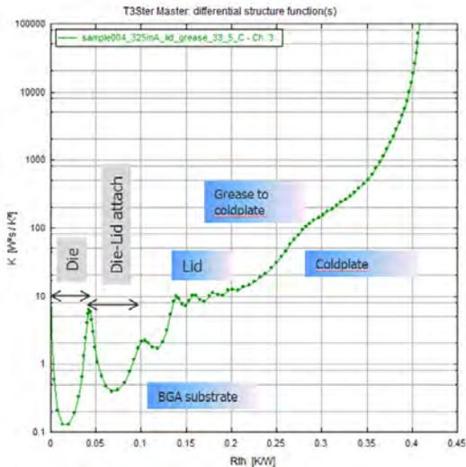
Figure 18. Baseline simulated structure functions in differential form
