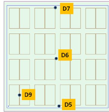
Figure 14. the locations of sensing diodes
