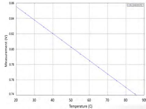
Figure 6. Thermal sensitivity (K factor)
