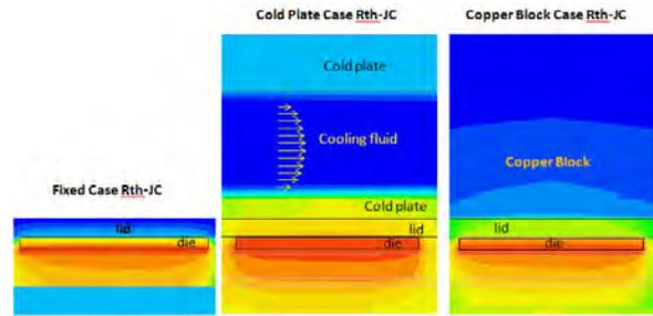
Figure 9. Temperature distributions near the die and lid
