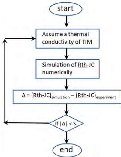
Figure 10. The simulation scheme to determine effective material properties of TIM
