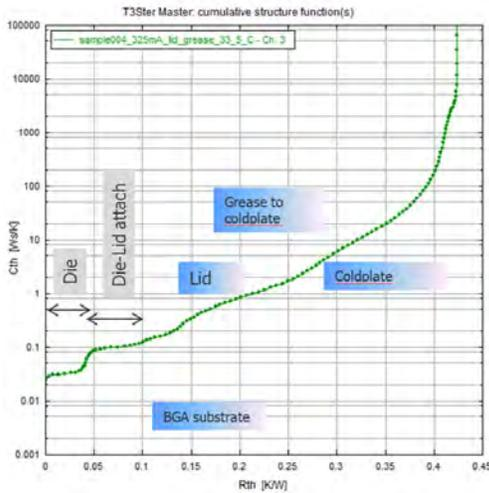
Figure 17. Baseline simulated structure functions in integral form
