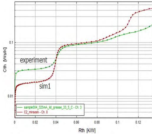
Figure 20. Experimental structure functions and baseline simulated structure functions near die region
