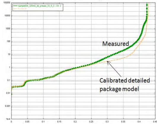
Figure 23. Experimental structure functions and final calibrated simulated structure functions
