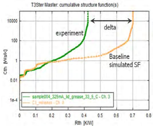
Figure 19. Experimental structure functions and baseline simulated structure functions
