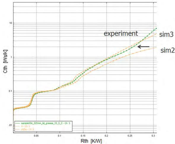
Figure 22. Experimental structure functions and calibrated simulated SFs structure functions
