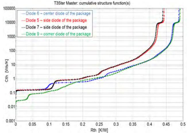
Figure 16. Experimental structure function curves
