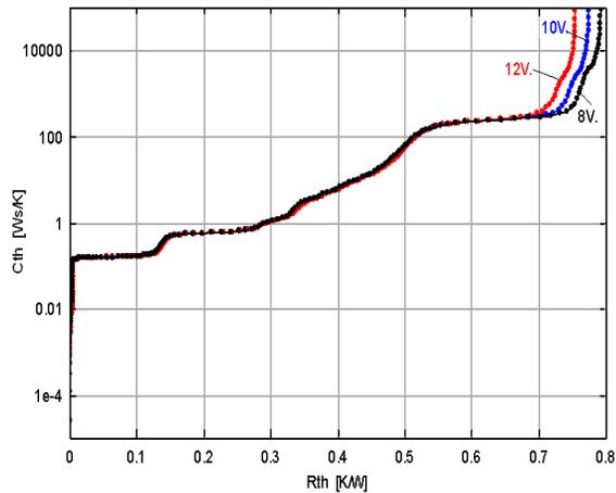
Figure 25. Measurement of thermal resistance of junction to ambient,  $R_{th-JA}$ , with various applied voltages on the fan
