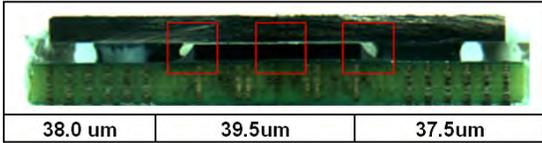
Figure 3. TIM thickness measurements
