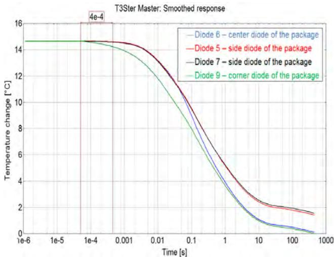
(b) Experimental temperature response curves with offset
