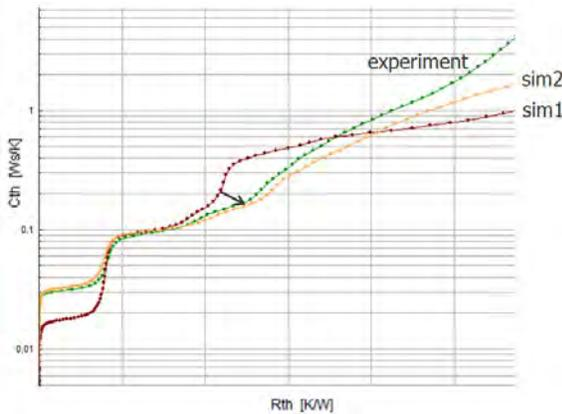
Figure 21. Experimental structure functions and calibrated simulated structure functions
