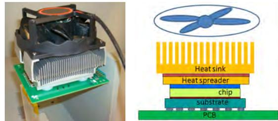
Figure 24. Forced convection fan cooling
