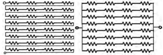
Figure 5. Serial and parallel resistor heater
