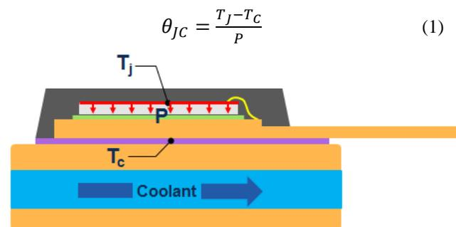
Figure 1: One-dimensional heat flow package.
