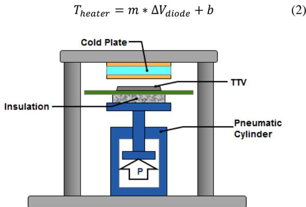
**Figure 4:** Theta JC test fixture.
