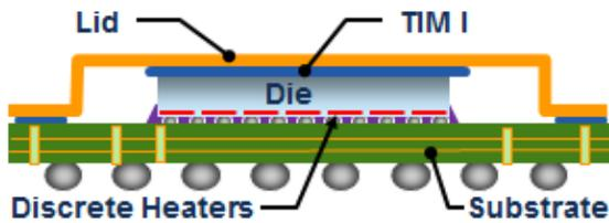
Figure 2: FCBGA Cross-section.
