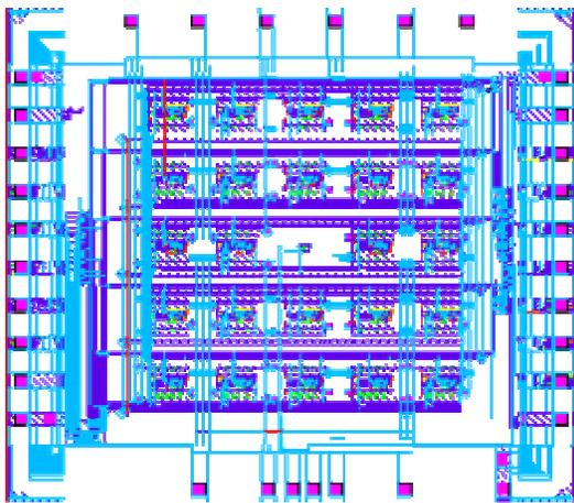
Figure 12. Layout diagram of the THBII thermal benchmark chip with an array of dissipator and temperature sensor cells and a temperature sensor diode in the middle
