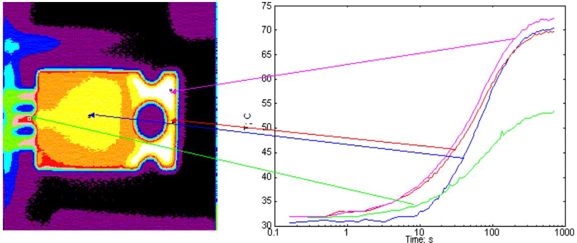
Figure 2. Thermal transients on the surface of the package of a power BT, recorded using IR thermography
