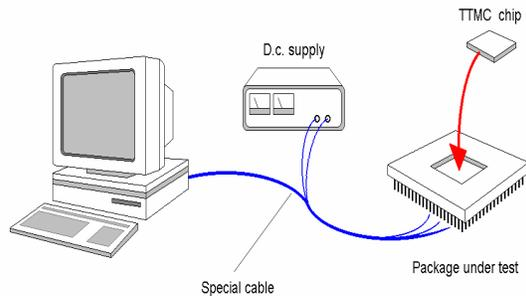
Figure 5. Arrangement for thermal transient measurement "without a tester"
