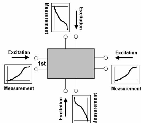
Figure 4. Both excitation and measurement are carried out on every port
