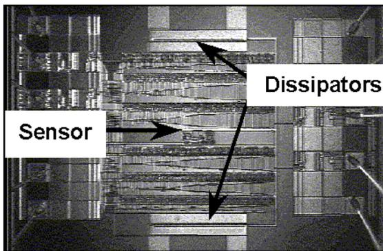
Figure 6. The present test chip of TTMK
