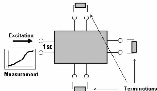
Figure 1. A method for the identification of a multi-port: both the excitation and the measurement are done on the primary port while the terminations on the further ports are varied
