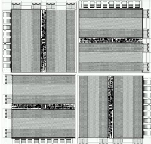
Figure 9. Tiling a large area with the new TTMC chip
