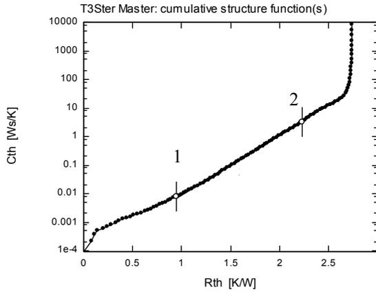
Figure 3: The cumulative structure function of homogeneous board.
