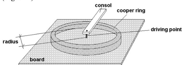
Figure 7: The board thermal conductivity measurement setup
