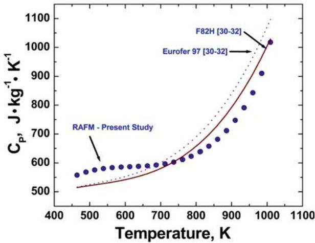
**Fig. 4** Comparison of  $C_p$  of the reduced activation steel (RAFM) estimated in this study from present drop calorimetry enthalpy measurements with the literature data on Eurofer 97 and F82H [30–32]
