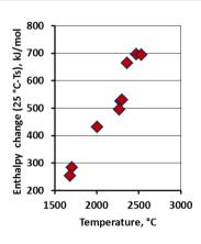
The figure shows drop enthalpies on four  $Y_2O_3$  samples 30-40 mg in weight.
