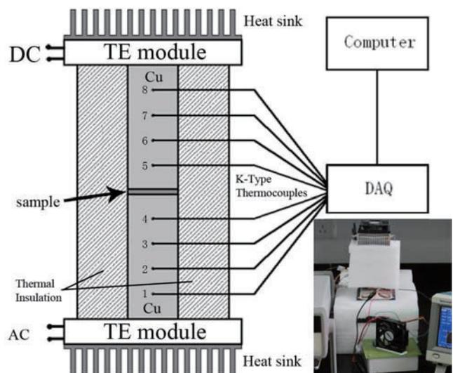
Figure1. Schematic and photography (insert) of experimental apparatus
