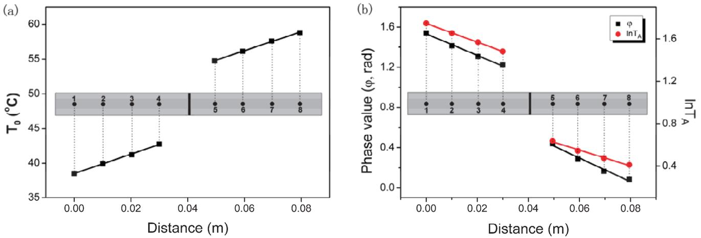
Figure 4. Distribution of (a) equilibrium temperature  $T_0$  and (b) phase value  $\phi$  and nature logarithm of temperature amplitude  $\ln T_A$  along the cylinders. Location 1 was considered as origin point. The specimen was PTFE with thickness of 112  $\mu\text{m}$ . The upper TE module was applied by 10V DC voltage and served as plate heater. The lower TE module was input by AC voltage with peak-to-peak voltage of 10 V and frequency of 5 mHz.
