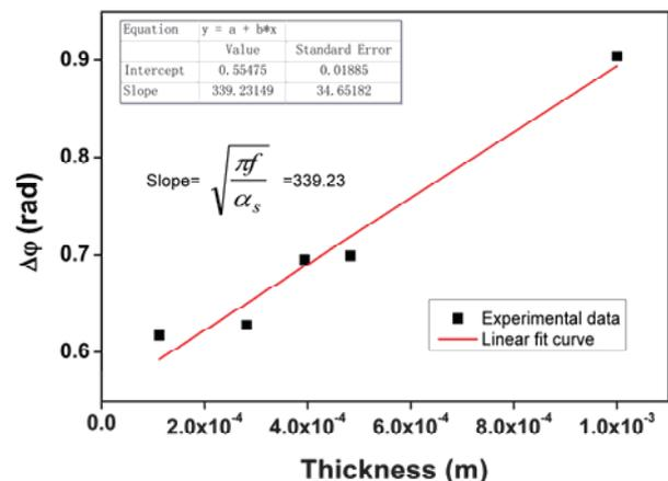
Figure 6. Phase difference vs. thickness of specimens
