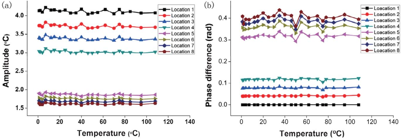
Figure 3. Tendency of (a) amplitude of temperature oscillation and (b) phase difference under different temperature at the contact surface between upper TE module with cylinder. The temperature was controlled by varying the voltage of upper TE module. AC voltage with peak-to-peak voltage of 10 V and frequency of 5 mHz was applied on the lower TE module.
