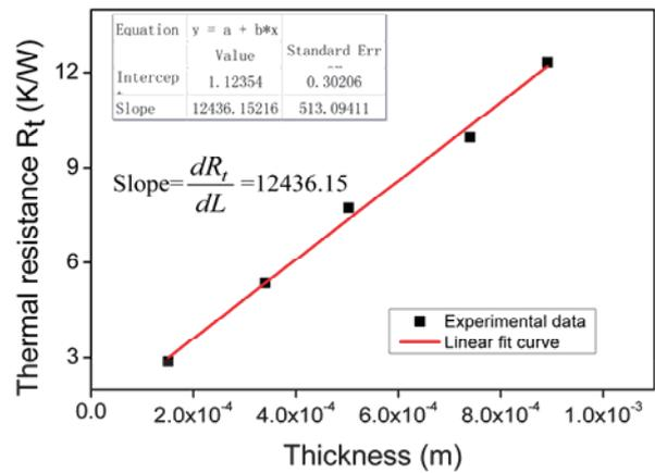
Figure 5. Thermal resistance vs. thickness of specimens
