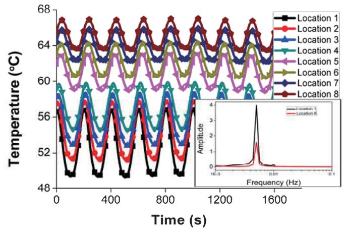
Figure 2. Temperature fluctuation at each thermocouple measuring location without specimen. Insert is FFT of temperature fluctuation at location 1. DC voltage of 8 V was placed on the upper TE module and AC voltage with peak-to-peak voltage of 10 V and frequency of 5 mHz was applied on the lower TE module.
