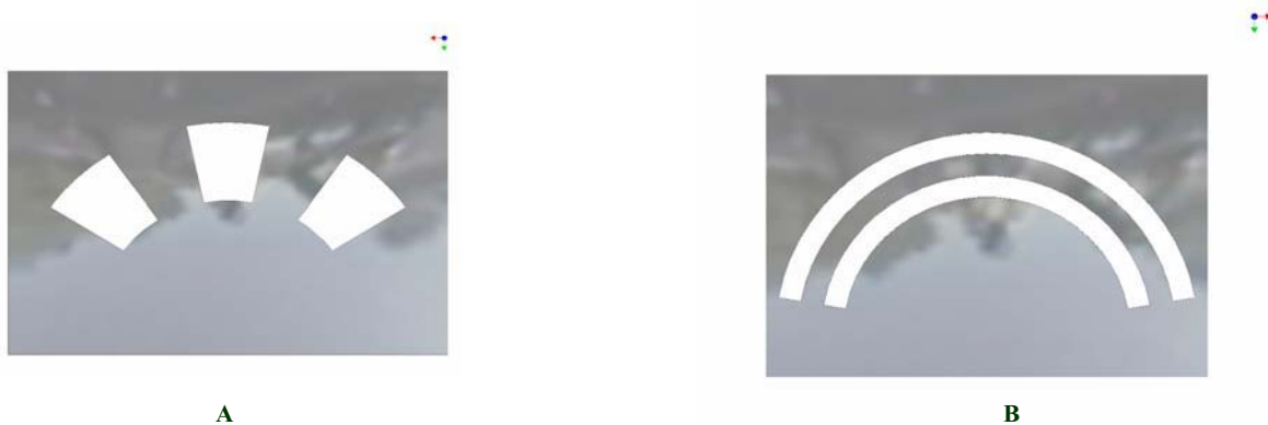
Figure 3. A) Mask for circumferential diffusivity ( \alpha_x ) measurement of C/C disk, B) Mask for radial diffusivity ( \alpha_y ) measurement of C/C disk.
