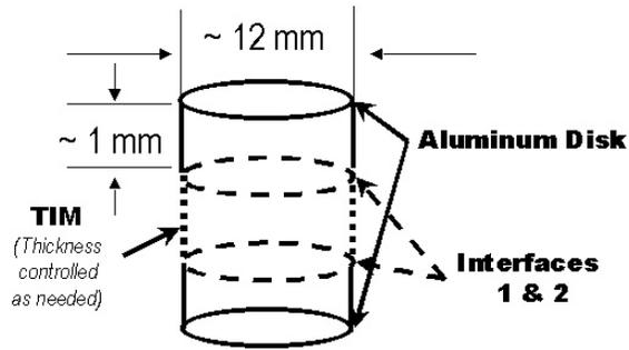
Figure 2. Preparation of specimen for thermal measurements.
