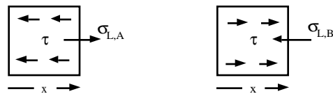
Figure D.2 – Free body diagrams of cylindrical shells A and B.
