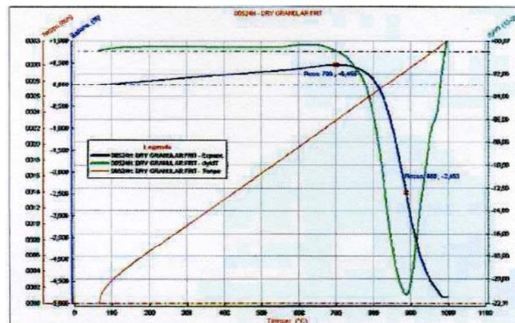
Fig. 8 Thermal expansion and sintering of an incoherent granular frit (blue curve), derivative (green), time (red).
