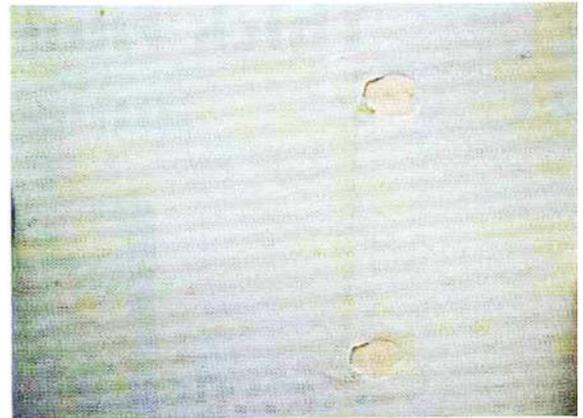
Fig. 15 Experimental method to collect the glaze layer as applied on the glaze line. A small piece of ashless laboratory filter is set on the tile before the application. After the application it is visible the relief given by the paper under the glaze.
