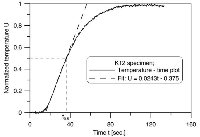
Fig. 12. Normalized temperature versus time at the rear surface for K12 specimen
