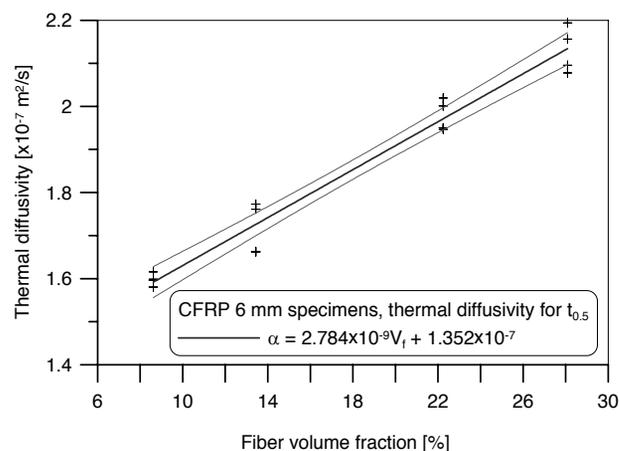
Fig. 14. Thermal diffusivity of CFRP composites with different fiber content [15]
