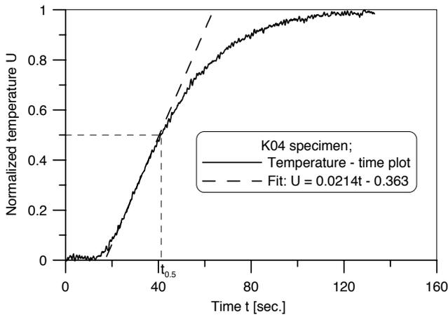
Fig. 8. Normalized temperature versus time at the rear surface for K04 specimen
