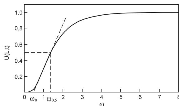
Fig. 1. Dimensionless plot of rear surface temperature history [17]
