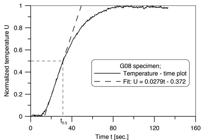
Fig. 4. Normalized temperature versus time at the rear surface for G08 specimen
