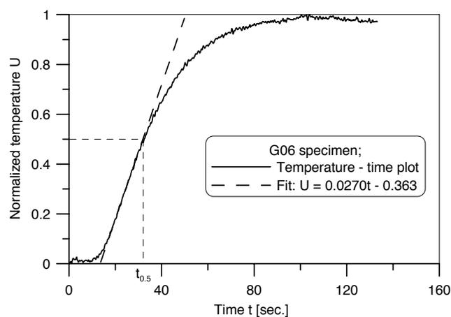
Fig. 3. Normalized temperature versus time at the rear surface for G06 specimen
