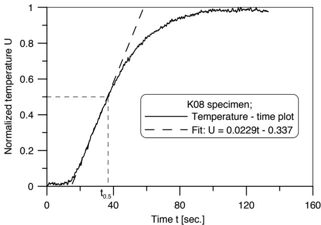
Fig. 10. Normalized temperature versus time at the rear surface for K08 specimen
