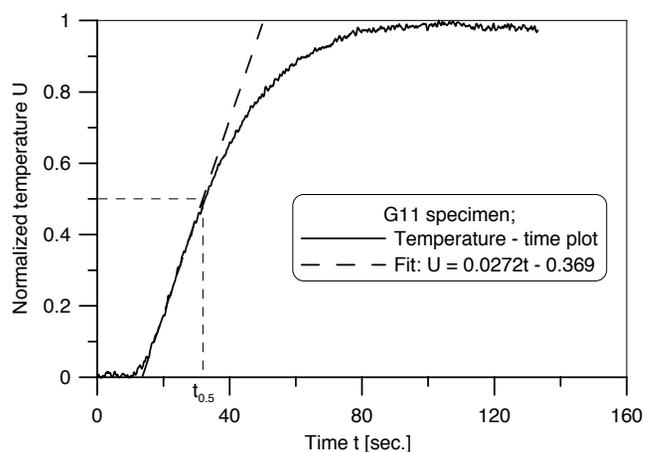
Fig. 6. Normalized temperature versus time at the rear surface for G11 specimen
