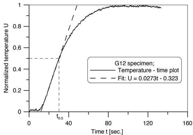
Fig. 7. Normalized temperature versus time at the rear surface for G12 specimen
