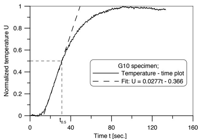
Fig. 5. Normalized temperature versus time at the rear surface for G10 specimen
