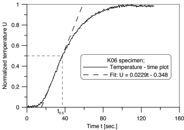
Fig. 9. Normalized temperature versus time at the rear surface for K06 specimen
