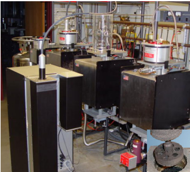
Fig. 1 Laser flash diffusivity system, Anter FL5000 with a 6-sample carousel
