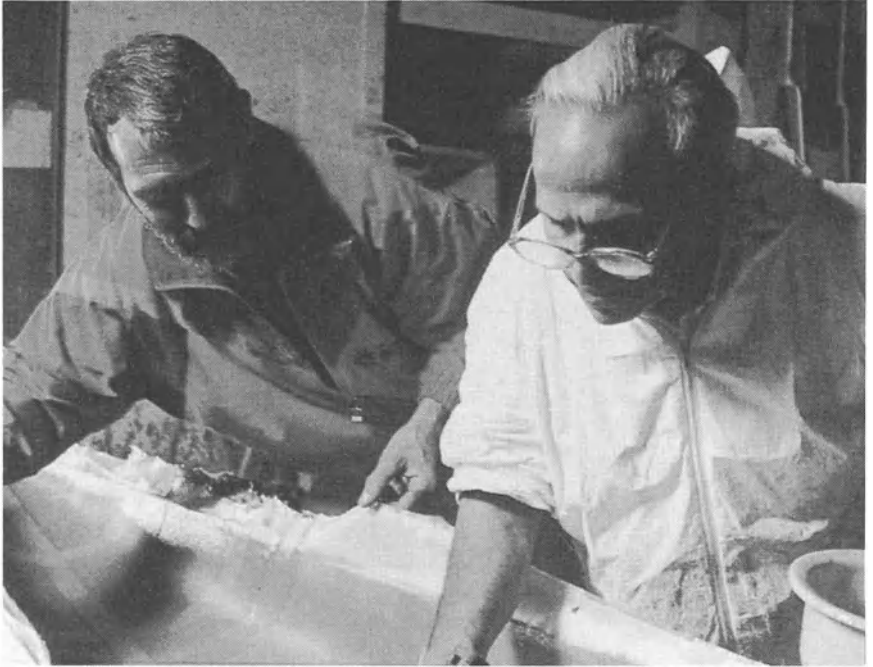
Fig. 4.12 Hand lay-up of a Kevlar/carbon fabric reinforced racing kayak using GRP tooling (courtesy Gaybo International Ltd.).
