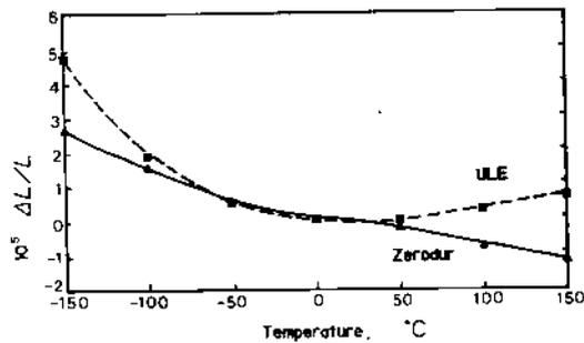
Fig. 5. Linear thermal expansion  $\Delta L/L$  of ULE and Zerodur. The symbols  $\blacksquare$  and  $\blacktriangle$  are these average values from three different dilatometers. The curves — and --- are merely a guide to the eye.
