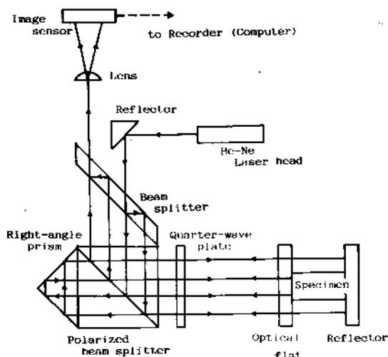
Fig. 2. Optical arrangement of the Type II dilatometer.
