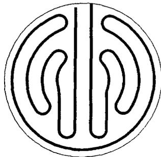
Figure 5 - *Re-designed heater layout in meter plate.*
