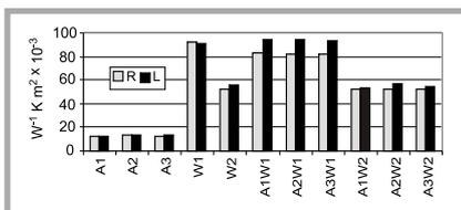
Figure 7. The thermal resistance of the textile materials.
