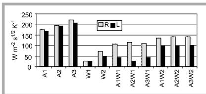
Figure 6. The thermal absorption of the textile materials.
