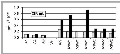
Figure 4. The thermal diffusion of the textile materials.
