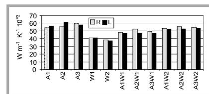
**Figure 2.** The thermal conductivity of the textile materials.
