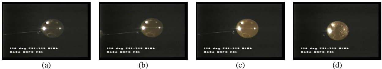
Figure 4. Triggered nucleation of \text{Ni}_{60}\text{Nb}_{40} a) pre trigger, b) trigger, c) 1s post trigger, d) 15s post trigger.
