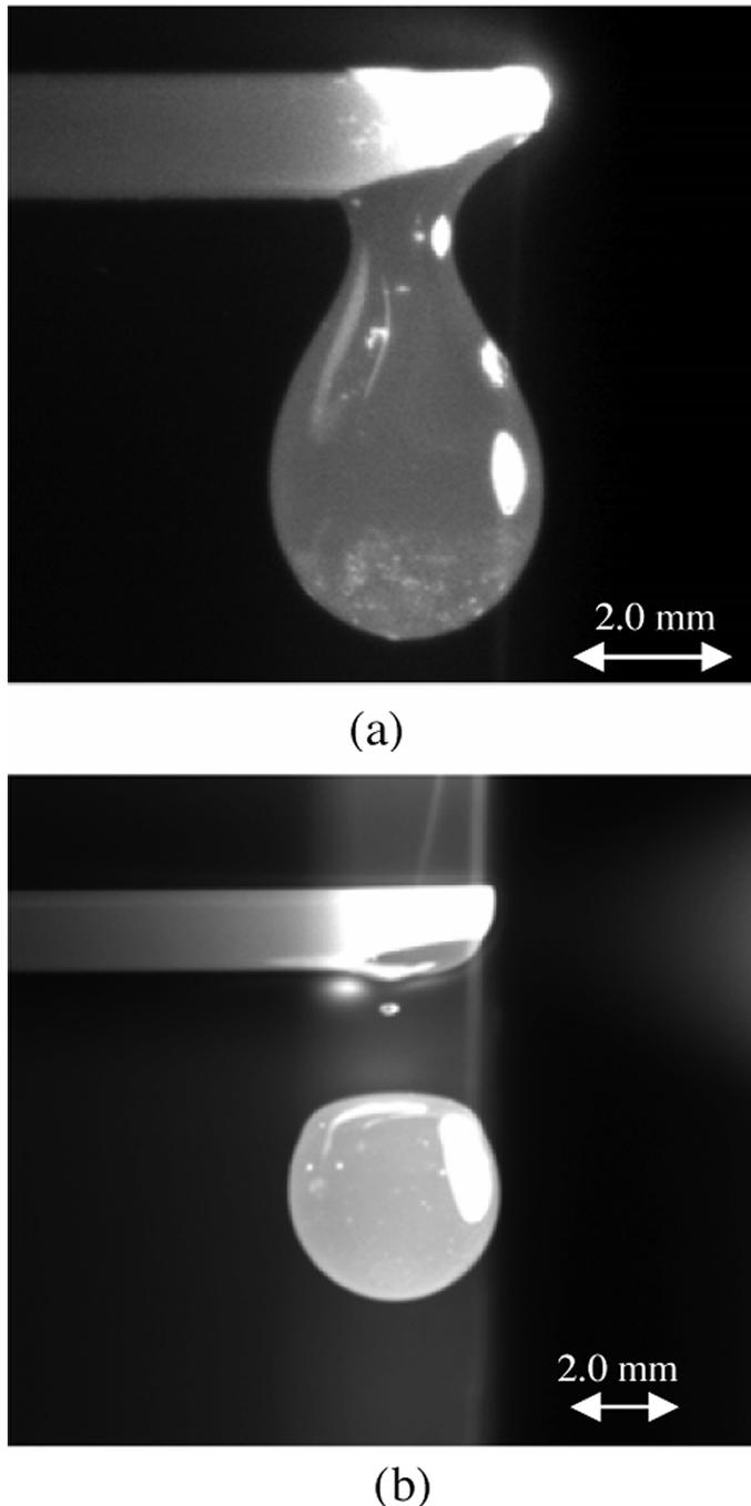
Fig. 2. (a) Symmetric pendant droplet of copper. (b) Detached drop and satellite droplet just after breakup.
