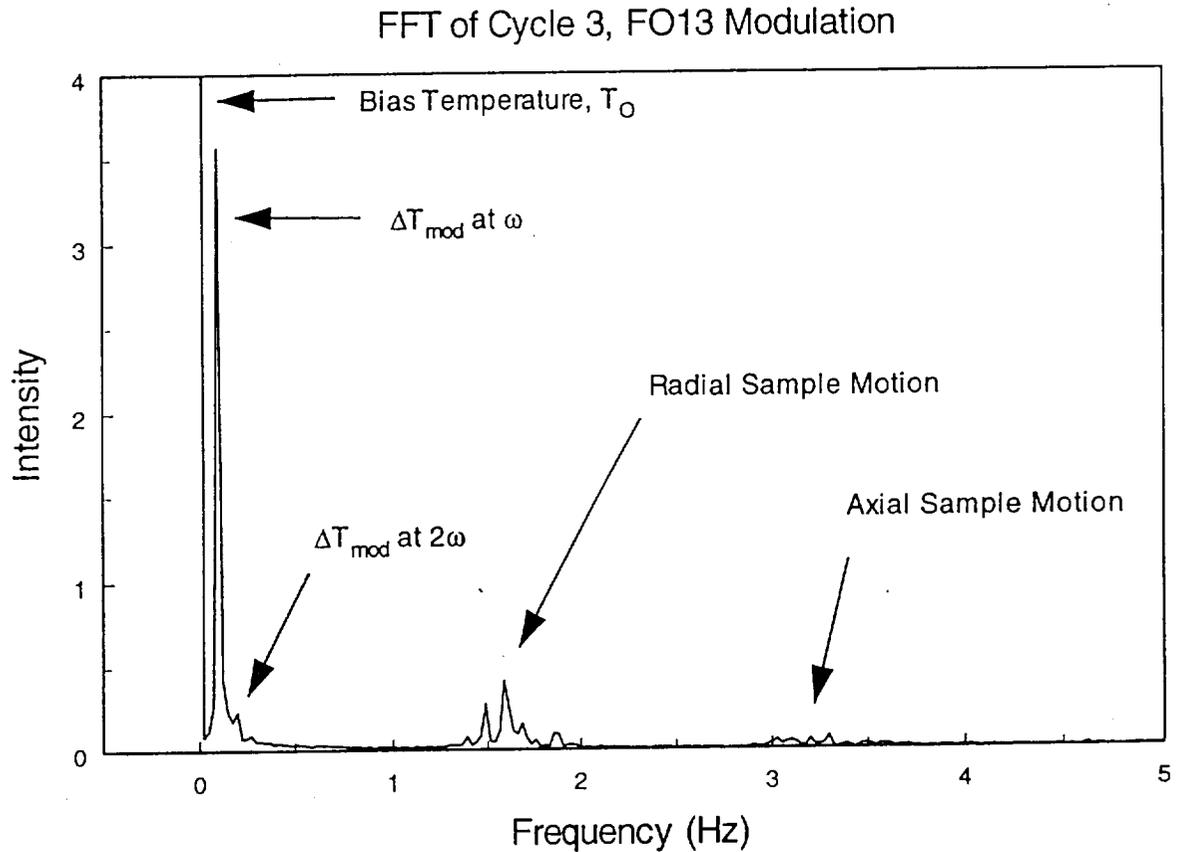
Figure 3. FFT spectrum of a NiNb modulation cycle.
