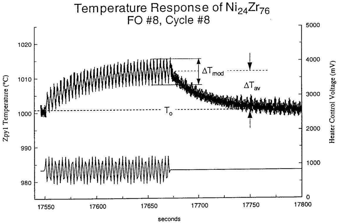
Figure 2. Temperature response of Ni<sub>24</sub>Zr<sub>76</sub> sample to RF power modulation.
