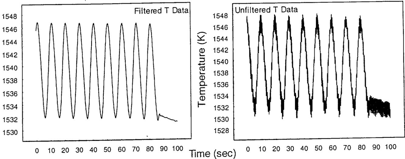
Figure 4a. Filtered data after applying 12th order Butterworth. The sample is  $Ni_{60}Nb_{40}$  and the modulation frequency is 0.1Hz (the corresponding FFT spectrum is shown in Figure 3). Note the slight phase shift in the signal (compare to 4b) resulting from the filter.
