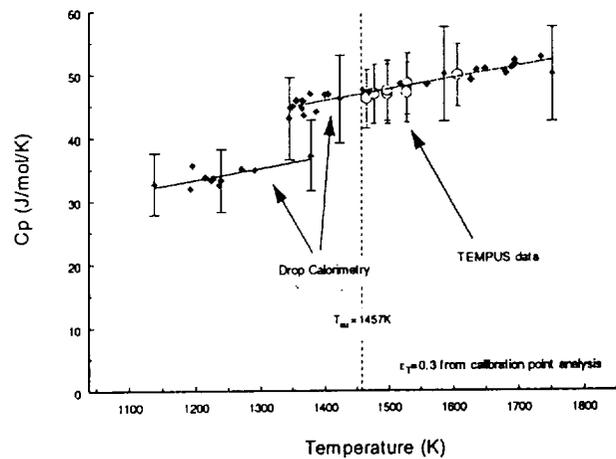
Figure 5. Drop calorimetry data plotted with data from IML-2.
