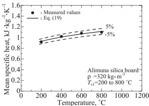
**Fig. 11.** Mean specific heat of alumina silica board: (●) measured values; (—) least squares fit of the measured results; (---)  $\pm 5\%$  deviations from the solid line.
