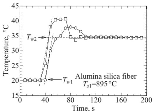
**Fig. 1.** Example of mean specific heat measurement.  $T_{w1}$  and  $T_{w2}$  are the water temperatures before and after dropping the specimen.
