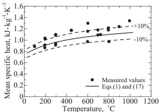
**Fig. 7.** Mean specific heat of the standard specimen SRM 720 Synthetic Sapphire ( $\alpha$ - $\text{Al}_2\text{O}_3$ ): (●) measured values; (—) Standard values by NIST; (---)  $\pm 5\%$  deviations from the solid line.
