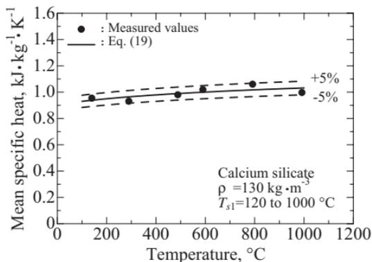
**Fig. 12.** Mean specific heat of calcium silicate: (●) measured values; (—) least squares fit of the measured results; (---)  $\pm 5\%$  deviations from the solid line.
