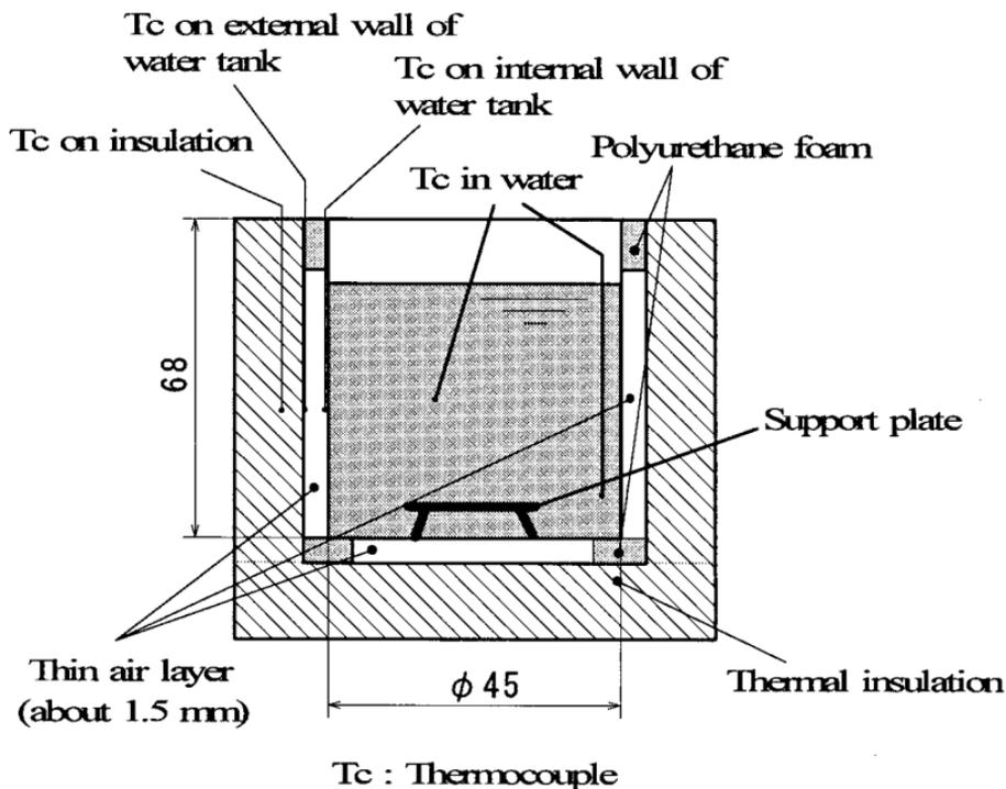
Fig. 3. Schematic of water tank for mean specific heat measurement. Dimensions in mm.
