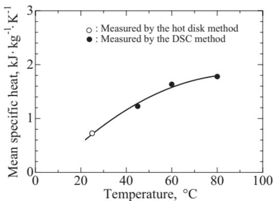
Fig. 4. Mean specific heat of paper used for water tank and support plate: (○) measured by the hot disk method; (●) measured by the DSC method; (—) least squares fit of the measured results.
