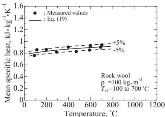
**Fig. 9.** Mean specific heat of rock wool: (●) measured values; (—) least squares fit of the measured results; (---)  $\pm 5\%$  deviations from the solid line.
