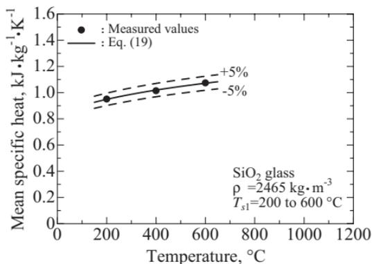
**Fig. 13.** Mean specific heat of  $\text{SiO}_2$  glass: (●) measured values; (—) least squares fit of the measured results; (---)  $\pm 5\%$  deviations from the solid line.
