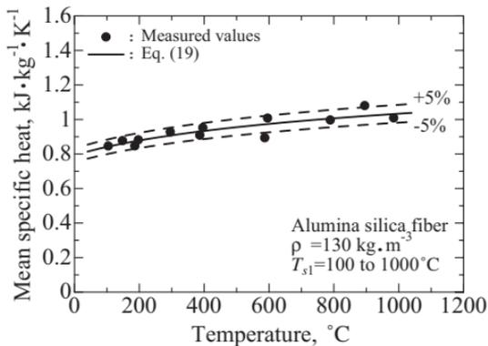
**Fig. 10.** Mean specific heat of alumina silica fiber: (●) measured values; (—) least squares fit of the measured results; (---)  $\pm 5\%$  deviations from the solid line.
