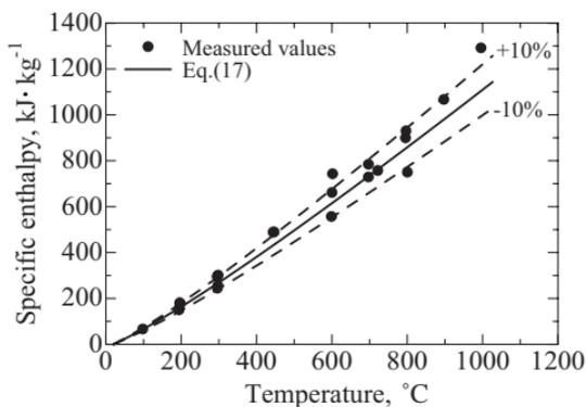
**Fig. 6.** Specific enthalpy of the standard specimen SRM 720 Synthetic Sapphire ( $\alpha$ - $\text{Al}_2\text{O}_3$ ): (●) measured values; (—) Standard values by NIST; (---)  $\pm 5\%$  deviations from the solid line.
