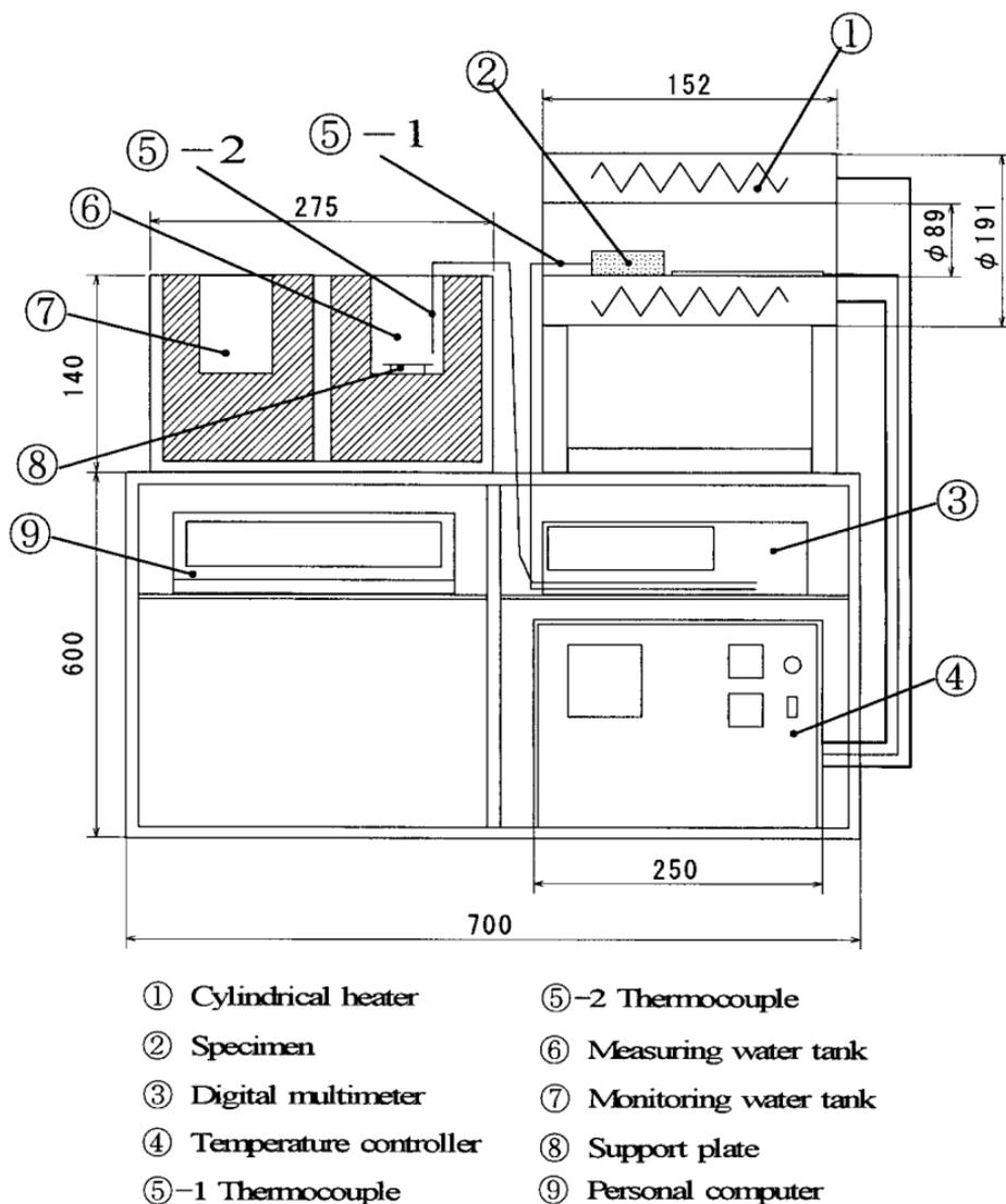
Fig. 2. Schematic of mean specific heat measuring apparatus. Dimensions in mm.
