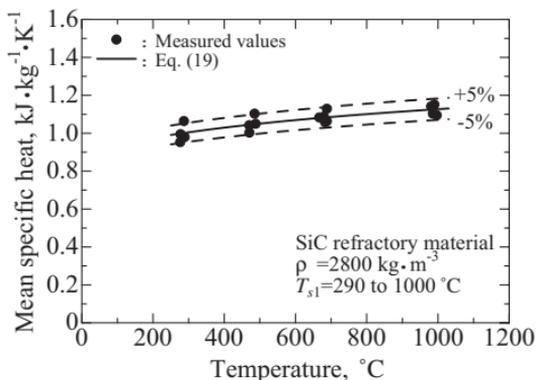
**Fig. 8.** Mean specific heat of SiC refractory material: (●) measured values; (—) least squares fit of the measured results; (---)  $\pm 5\%$  deviations from the solid line.
