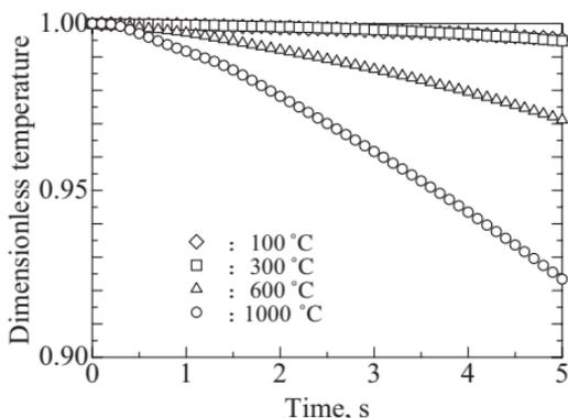
Fig. 5. Transient temperature change of a sample cube in air (Temperature at the center of the cube): ◇, □, △, ○ are the measured values at initial specimen temperatures of 100, 300, 600, 1000 °C, respectively.
