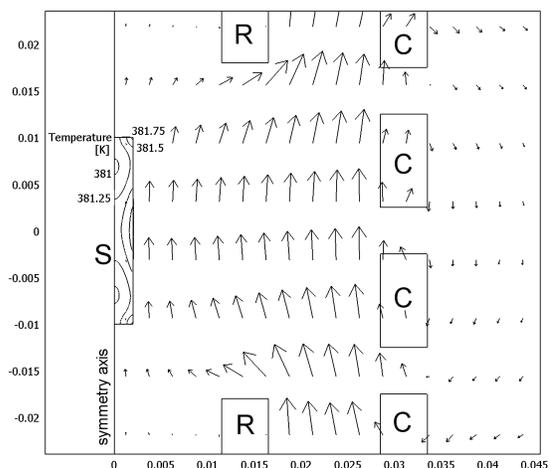
**Figure 3.** Temperature field of the specimen of Fig. 2 with temperature differences reduced by robber rings, computed with a FEA model; S – specimen, C – windings of the heating coil, R – robber rings
