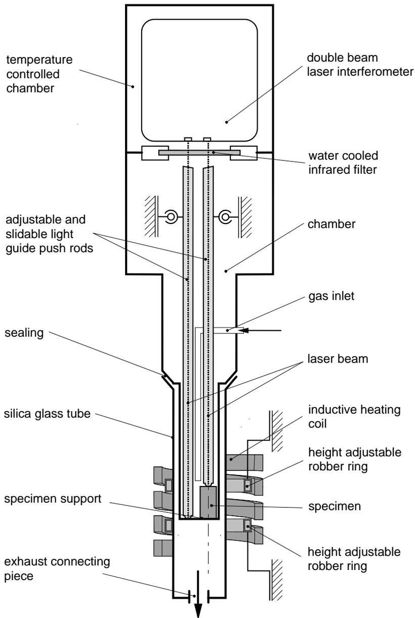
**Figure 1.** Schematic of the interferometric dilatometer with inductive heating of the sample
