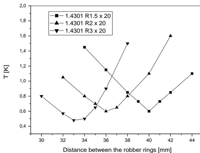
**Figure 5.** Temperature difference along the outer side of a cylindrical specimen  $\Delta T$  depending of the positions of the rubber rings  $P$
