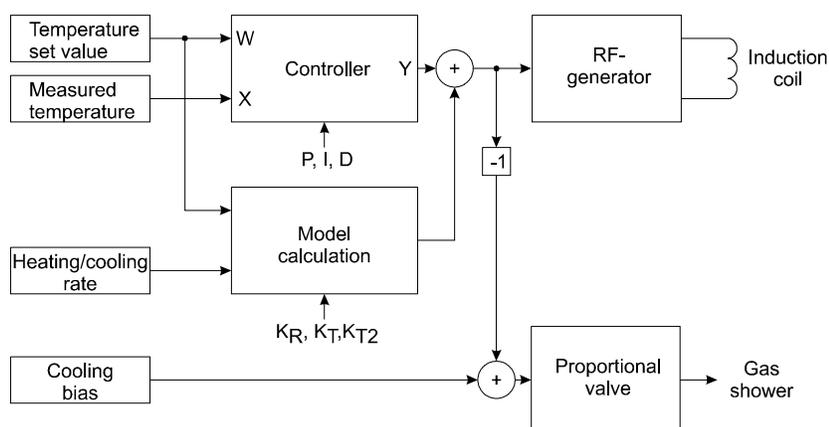
**Figure 7.** Block diagram of the control unit of the dilatometer
