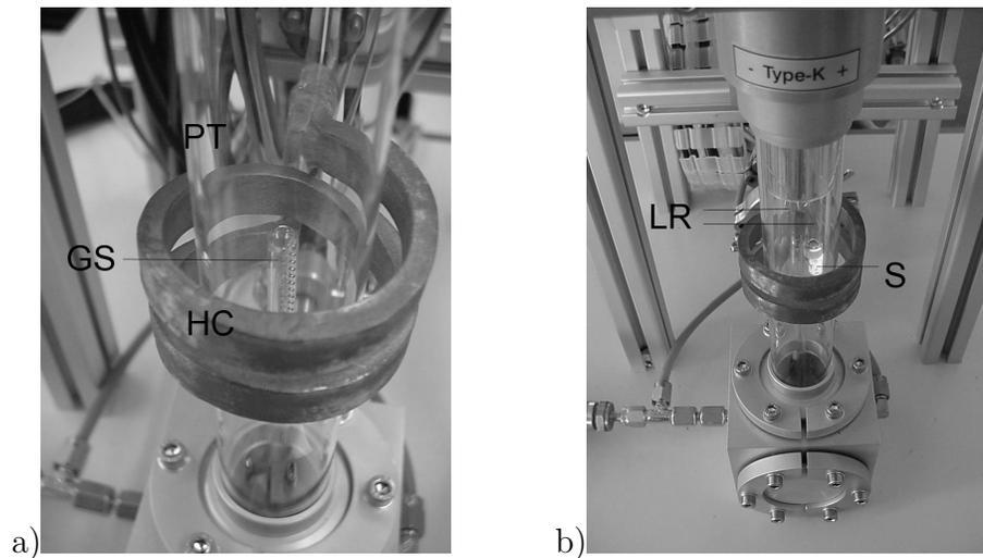
**Figure 6.** Sample holder and gas shower of the dilatometer, a) sample holder removed, PT – protection tube, HC – heating coil, GS – gas shower, b) sample holder in working position, S – sample, LR – light guide push rods
