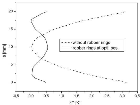
**Figure 4.** Temperature difference  $\Delta T$  along the outer side of a cylindrical specimen  $s$  with and without rubber rings, arrangement according to Fig. 2 and resp. Fig. 3
