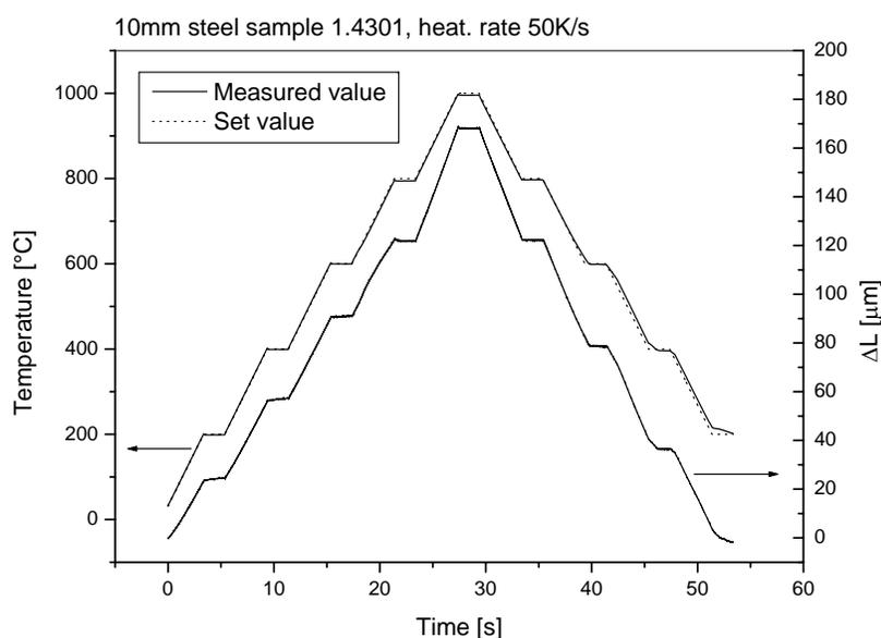
**Figure 8.** Nominal and measured temperature run of a specimen of stainless steel (1.4301) in form of a hollow cylinder (inner radius 4 mm, outer radius 6 mm, length 10 mm)
