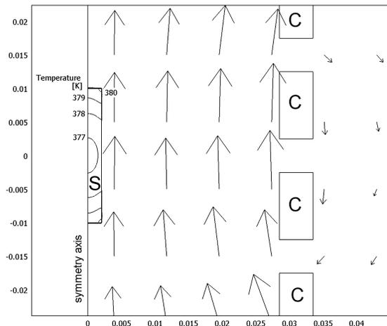
**Figure 2.** Temperature field of an inductively heated cylindrical (R2 x 20) 1.4301 steel sample, computed using a FEA model; S – specimen, C – windings of the heating coil
