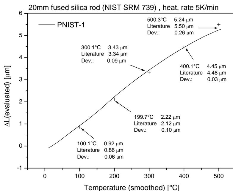
**Figure 9.** Measurement of a 20 mm fused silica rod, heating-rate 5 K/min
