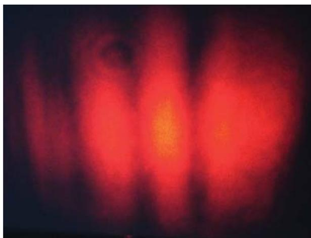
Fig. 2. Interference fringes obtained with the Michelson interferometer.
