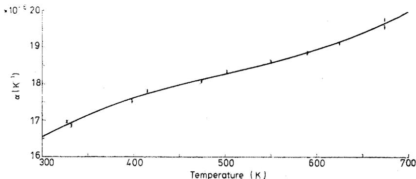
Figure 1. Measurements of the expansion coefficient of copper between 300 K and 700 K. Polynomial fit for  $\alpha$  is  $\alpha \times 10^6 = 6.818 + 5.639 \times 10^{-2} T - 1.001 \times 10^{-4} T^2 + 6.626 \times 10^{-8} T^3$ .
