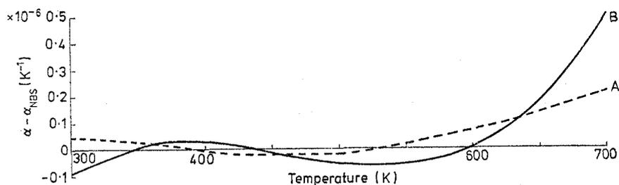
Figure 2. Differences from NBS calibration of SRM 736: A, Kollie *et al* (1973); B, this study.
