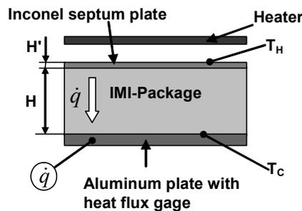
Figure 1: Schematic of the Thermal Conductivity Test Apparatus
