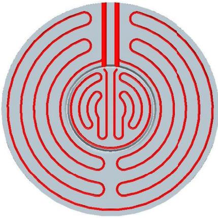
FIG. 5. The multiple heater layouts for the meter plate and guard plate.
