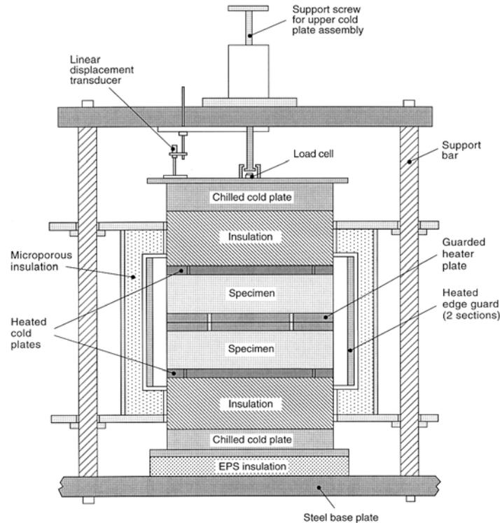
**Figure 3.** The NPL 305 mm diameter high temperature guarded hot-plate apparatus.
