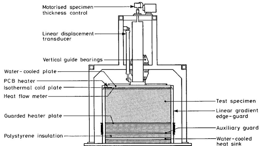
**Figure 2.** Essential features of the NPL 610 mm guarded hot plate/heat flow meter apparatus.
