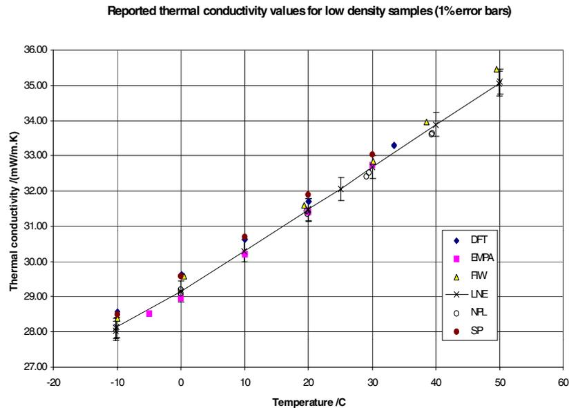
**Figure 4.** The thermal conductivity of IRMM-440 versus temperature over the range  $-10$  to  $+50$  °C.
