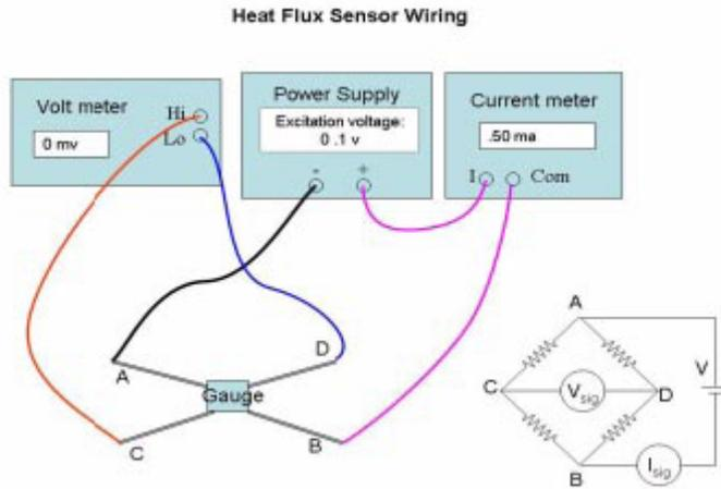
Figure 3. Wire connection with 2 meters
