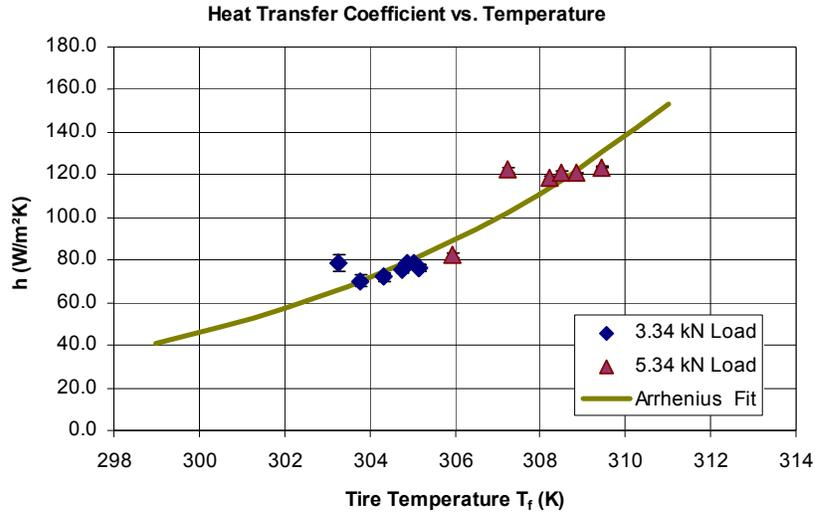
Figure 12: Heat Transfer (Film) Coefficient vs. Tire Temperature  $T_f$ .
