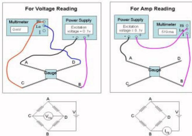
Figure 4. Wire connection with 1 meter
