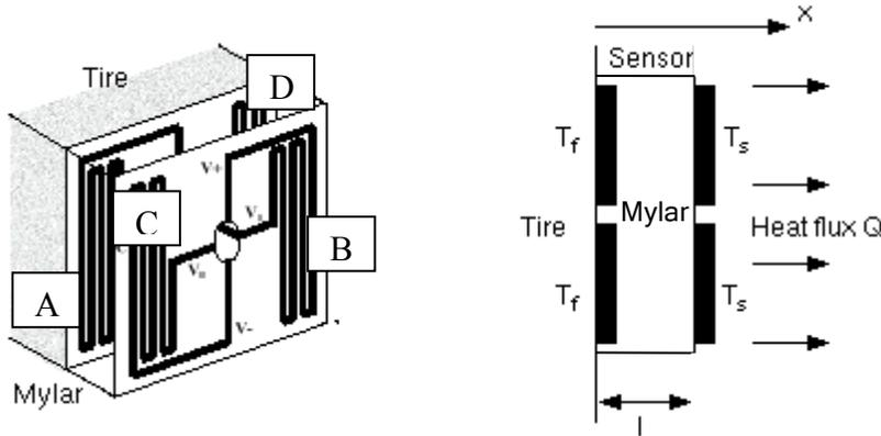
Figure 1. Double sided heat flux sensor schematic
