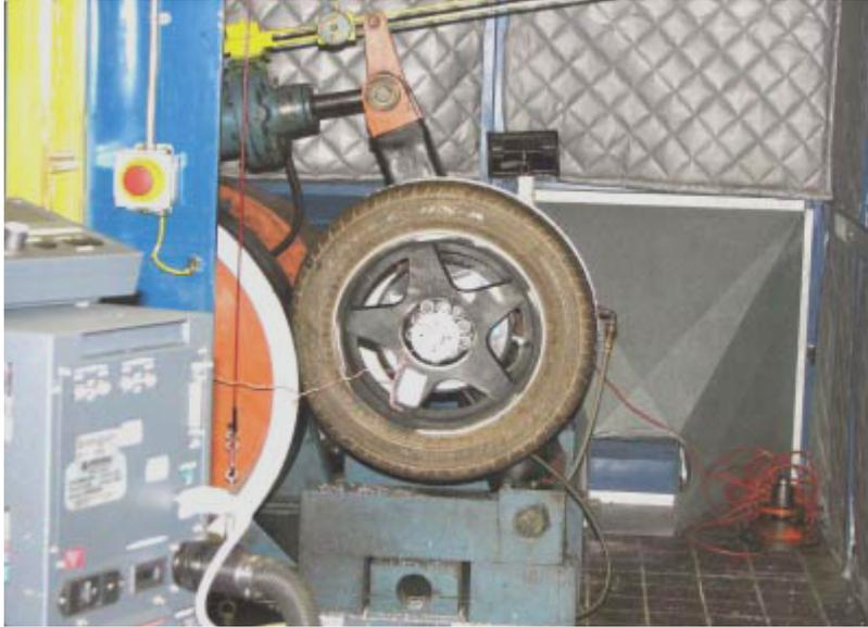
Figure 9. Sensor glued to rolling tire
