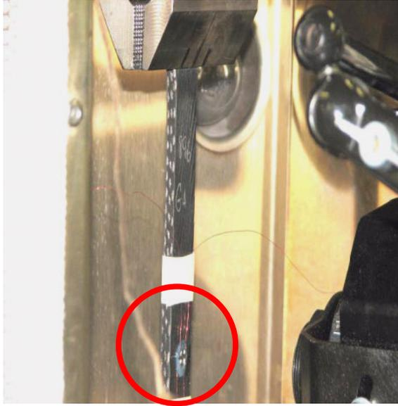
Figure 7. Heat flux sensor mounted on a 2-ply composite laminate
