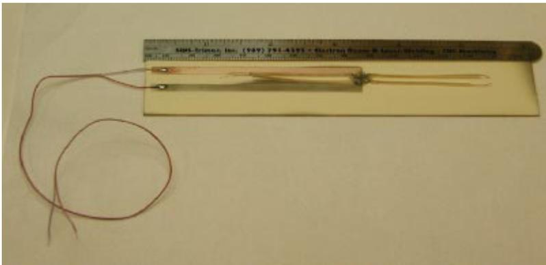
Figure 5. Combined thermocouple and heat flux sensor used for calibrating the bridge resistance vs. its temperature
