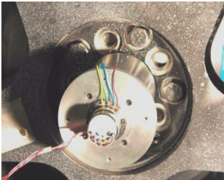
Figure 10. Lead wires attached to a slip ring
