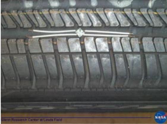
Figure 14. Heat flux sensor mounted on a passenger tire
