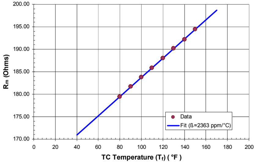
Figure 6. Calibration curve relating bridge resistance to its temperature
