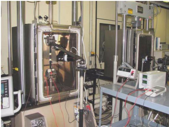
Figure 8. Connection of lead wires from the sensor to the power and reading meters
