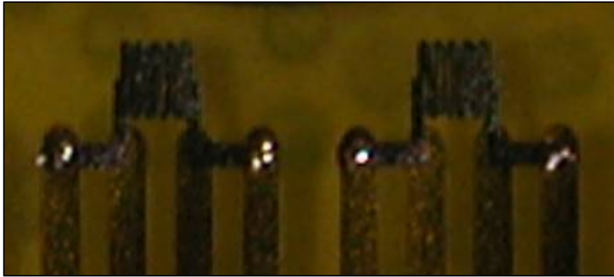
Figure 2 - Through-Holes of Current GTL Double-Sided Kapton Heat-Flux Gauge
