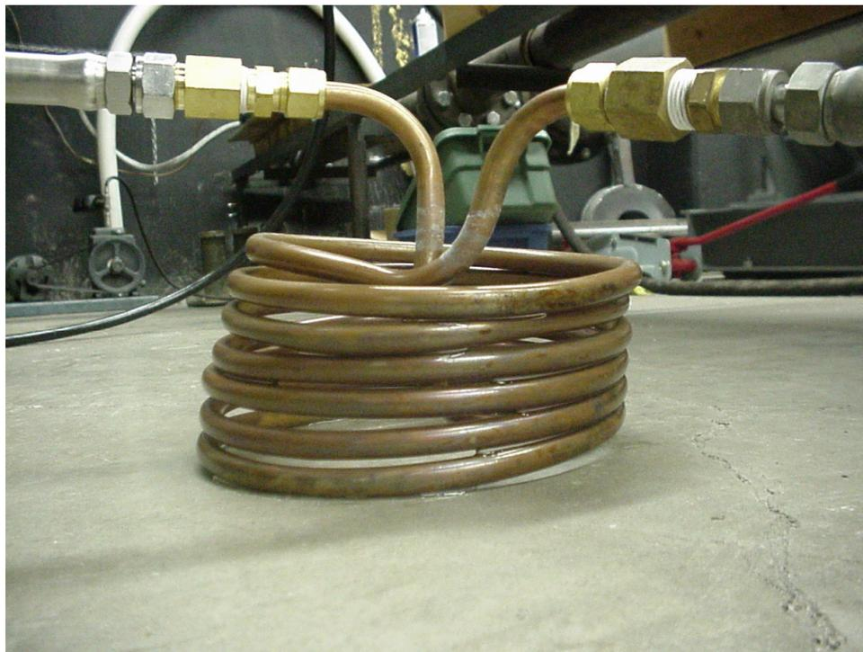
Fig. 4.5 Copper heat exchanger
