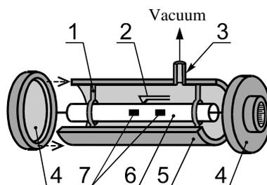
Fig. 3. Sketch of the test bench for the high-temperature calibration of the GHFS: 1) holder; 2) thermocouple; 3) tube for evacuating the system; 4) covers; 5) body; 6) tube; 7) GHFS to be calibrated.
