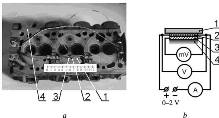
Fig. 2. Sketch of the calibration of the GHFS proposed in this paper: *a*) arrangement of the elements on the stand; *b*) basic circuit; 1) thermal insulation; 2) heater; 3) calibrated GHFS; 4) base.
