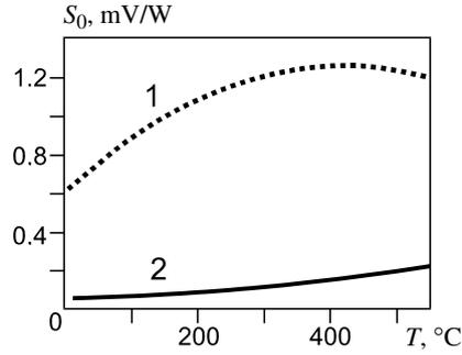
Fig. 4. Calibration curves for the GHFS: 1) 12N18Kh9T steel + nickel; 2) chromel + alumel.
