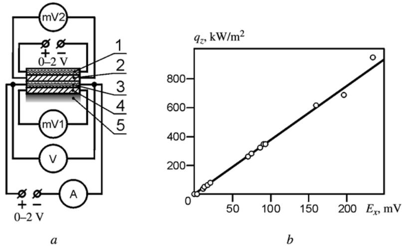
Fig. 1. Sketch of the calibration test bench (a) and the results of the calibration of a typical GHFS made of bismuth (b), where the points denote data obtained by an alternative method: 1) “guard” heater; 2) additional GHFS in the zero-indicator function; 3) heater; 4) calibrated GHFS; 5) base.
