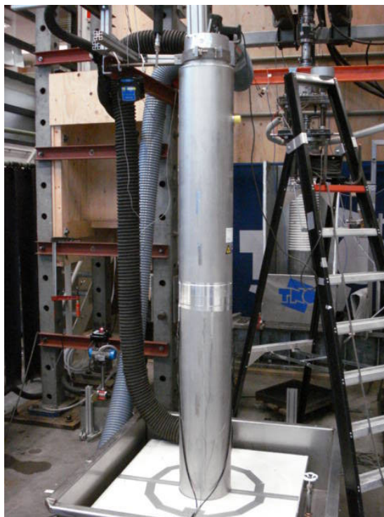
Figure 8. VI pipe erected vertically with HFT mounted. Shield removed.
